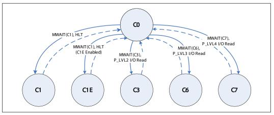
While individual threads can request low-power C-states, power saving actions only take place once the core C-state is resolved. Core C-states are automatically resolved by the processor. For thread and core C-states, a transition to and from C0 is required before entering any other C-state.
