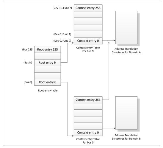
Figure 10. Device to Domain Mapping Structures
