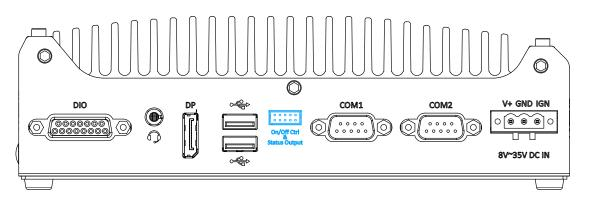
The "On/ Off Control Ctrl & Status Output" connection allows for external switch and LED indicator extension. It is useful when the system is placed in a cabinet or a not easily accessed location. This function is provided via a 2x5 2.0mm pitch wafer connector.
