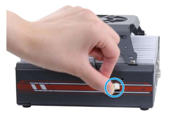
4. Once the power cable is connected, place the supplied cable cover (in the accessory box) over the cable and secure it with the screws indicated to complete the installation.
