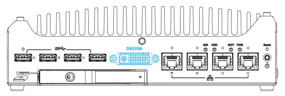
The system features a DVI-I connector on its front panel that is also compatible with VGA signals. The DVI and VGA outputs are directly driven by integrated Intel HD graphics engine and support up to 1920 x 1200 resolution.
