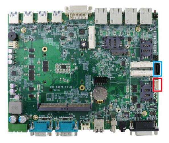
The system provides one SATA port which support Gen3, 6 Gb/s SATA signals. The SATA port is composed of a 7-pin SATA connector (indicated in blue) and a 4-pin power connector (indicated in red). This SATA and power connector should be pre-connected to the external 2.5" hot-swappable tray.
