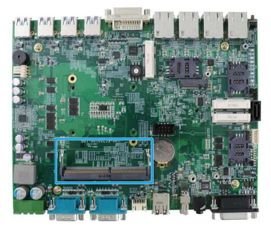
3. To install the memory module, insert gold fingers of the module into the slot at 45 degree angle, push down on the edge of the module and the clips on the side should clip the module into position.
