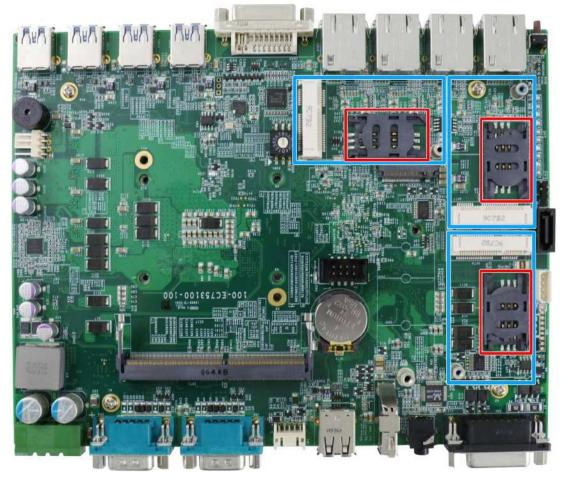
The system has three mini-PCIe sockets and there are plenty of off-the-shelf mini-PCIe modules with versatile capabilities. By installing a mini-PCIe module, your system can have expanded features such as WIFI, GPS, CAN bus, analog frame grabber, etc.
