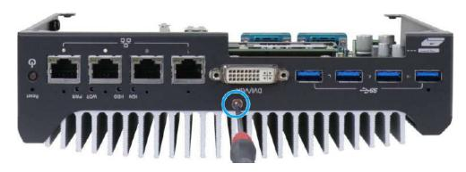
4. Remove the screws from the top of the heatsink and separate the motherboard/ heatsink from the enclosure.
