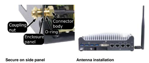
7. <u>Reinstall the system enclosure</u>, panel and external antenna.
