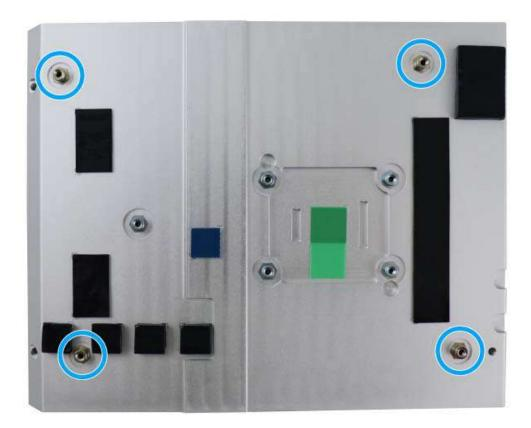
Secure the four (4) M3 P-head motherboard screws (indicated in blue) and from the accessory box, five (5) M3 spring screws (indicated in red). Gradually tighten the five screws in the following order for even pressure.
