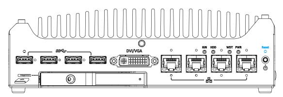
The reset button can be used to manually reset the system in case of abnormal condition. To avoid unexpected operation, the reset button is hidden behind the front panel. You need to use a pin-like object to push the reset button.
