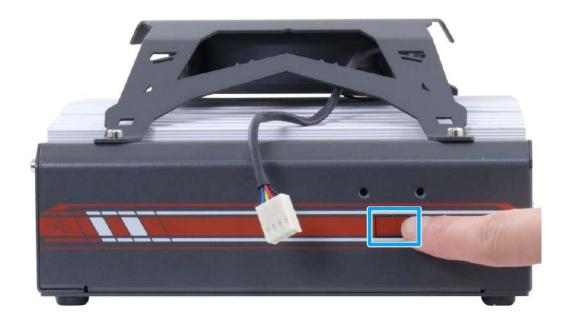
3. Connect the 4-pin fan's power cable to the 4-pin fan power connector.
