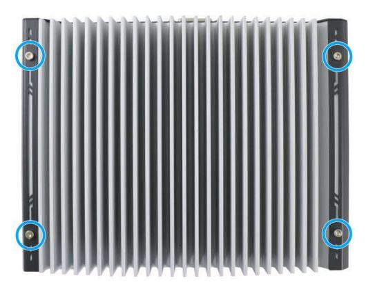
5. Turn the motherboard/ heatsink around to gain access to internal components and expansions.
