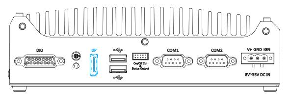
The system has a DisplayPort (DP) output which is a digital display interface that mainly connect video source and carry audio to a display device. When connecting a DP, it can deliver up to 4K UHD (4096 x 2304) in resolution. The system is designed to support passive DP adapter/ cable. You can connect to other display devices using DP-to-HDMI cable or DP-to-DVI cable.
