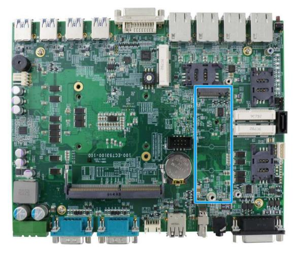
The system has an M.2 2280 slot (SATA signal only) for you to install an M.2 SATA SSD for faster access over traditional hard disk drives.
