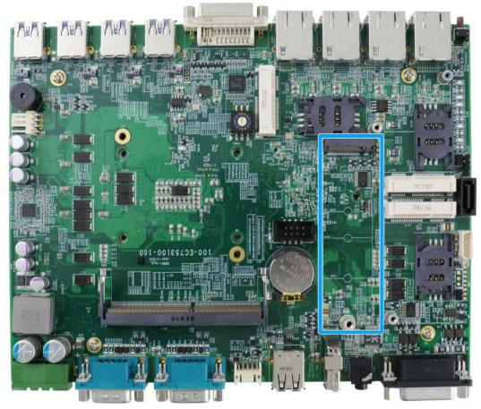
The system has an SATA signal M.2 2280 slot for you to install an M.2 2280 SATA SSD. For installation, please refer to the following instructions.
