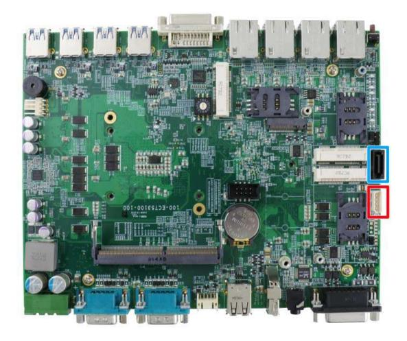
The system has one SATA port (blue) and one four pin power connector (red). The SATA and power cables should already be connected on the motherboard so users only need to install the 2.5" SATA HDDs/ SSDs to the front hot-swappable tray.
