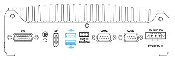
The system has two USB 2.0 ports. They are implemented by native xHCI (eXtensible Host Controller Interface) controller in H310 chipset and are compatible with USB 2.0, USB 1.1 and USB 1.0 devices. Legacy USB support is also provided so you can use USB keyboard/mouse in DOS environment.
