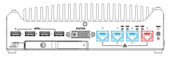
The system offers four GbE ports with screw-lock mechanism. The GbE port marked in red is implemented with Intel® I219-LM while the ones marked in blue and are implemented with Intel<sup>®</sup> I210-IT controllers. Each port has one dedicated PCI Express link for maximum performance. When an Ethernet connection is established, the LED indicators on the RJ45 connector represents the following connection statuses:
