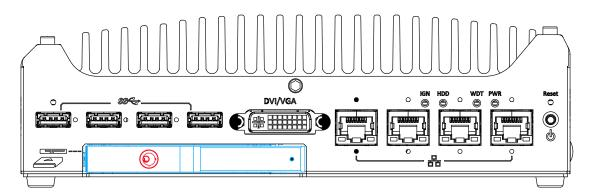
The system features an external hot-swappable 2.5" hot-swappable tray that supports a 7mm or 9.5mm 2.5" HDD/ SSD. The 7mm HDD/ SSD will need attach PORON materials supplied to make up for the thickness difference. Designed for easy access, the HDD tray is secured by a lock (indicated in **red**).
