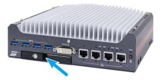
4. If you are installing a 7mm thickness HDD/ SDD, please attach the PORON materials supplied, at the corners of the non-label side, on the HDD/ SSD. With the label side facing upward, insert the SATA connector side of the 2.5" HDD/ SSD into the slot first. You may feel resistance when the SATA connectors meet, push it in firmly until the 2.5" HDD/ SSD is fully inserted into the slot.
