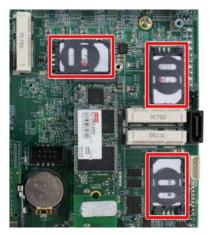
Secure the SIM card by sliding the holder
