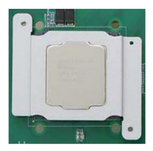
6. Turn the motherboard around and secure the bracket by tightening two M3 P-head screws.
