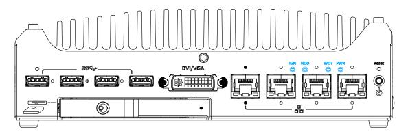
There are four LED indicators on the I/O panel: PWR, WDT, HDD and IGN. The descriptions of these LEDs are listed in the following table.
