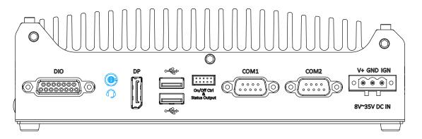
There is a female 4-pole audio jack for headphone (speaker) output and microphone input. To utilize the audio function in Windows, you need to install corresponding drivers. Please refer to the section, <u>Driver Installation</u>.
