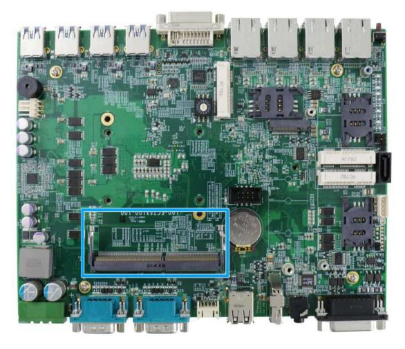
The system motherboard supports one 260-pin SODIMM socket for installing one DDR4-2666/ 2400 memory module up to 32GB capacity.
