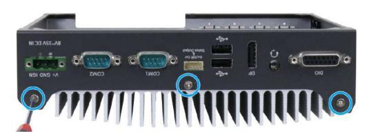
4. Secure the six screws at the bottom to complete enclosure installation process.
