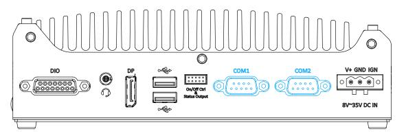
The system provides two COM ports for communicating with external devices. These COM ports are implemented using industrial-grade ITE8786 Super IO chip (-40 to 85°C) and provide up to 115200 bps baud rate.
