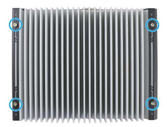
2. Secure the screw on the front I/O panel to the heatsink.
