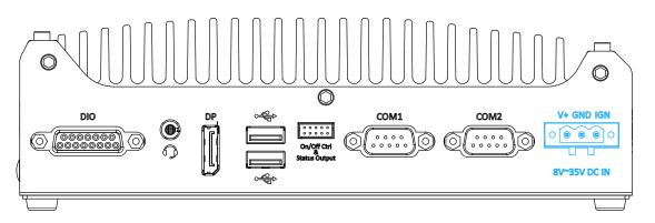
The system accepts a wide range of DC power input from 8 to 35V via a 3-pin pluggable terminal block, which is fit for field usage where DC power is usually provided. The screw clamping mechanism on the terminal block offers connection reliability when wiring DC power.
