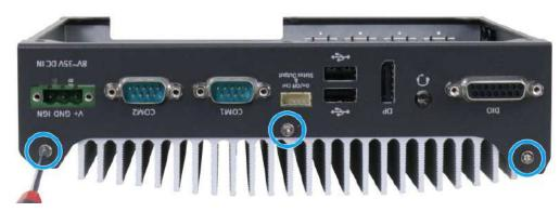
3. Remove the screws indicated on the front I/O panel.
