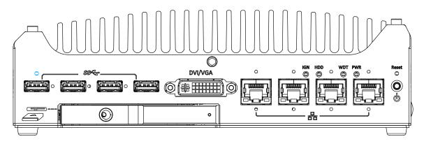
The CMOS Reset button is used to manually reset the motherboard BIOS in case of system halt or malfunction. To avoid unexpected operation, it is purposely placed behind the panel. To reset, please use the tip of a pen, press and hold for at least 5 seconds to reset the BIOS.
