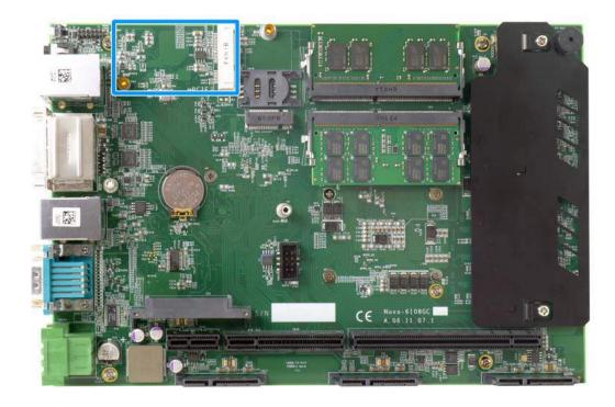
The system has a mini-PCIe slot (indicated in **blue**) for installing WiFi module. For installation, please refer to the following instructions.
