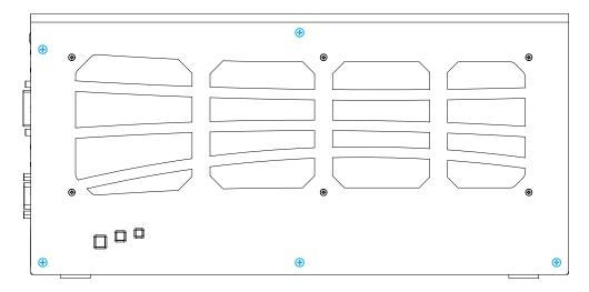
5. Secure screws on the ventilation fan panel highlighted in **blue** to complete the enclosure installation process.
