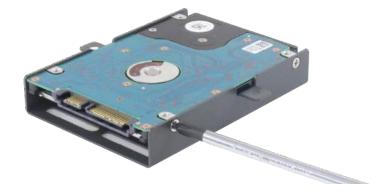
Gently insert the SATA port of HDD/ SSD to SATA port 1, the two screw hole should meet the standoffs on the motherboard, screw using two M3 P-head screws.
