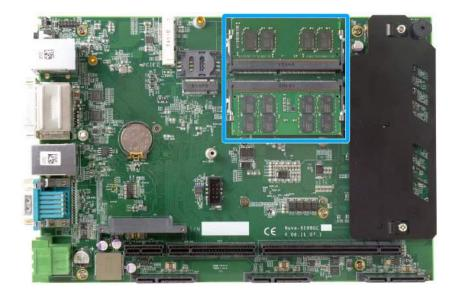
There are two memory SO-DIMM slots on the motherboard that support a total maximum of 32GB DDR4-2133. Please follow the procedures below to replace or install the memory modules.
