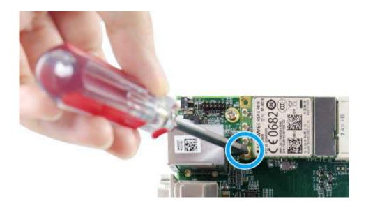
4. Clip on the IPEZ-to-SMA cable to the module and secure the antenna to the rear panel. Please refer to the module's manual for clip-on connection.
