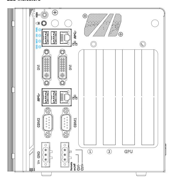
There are four LED indicators on the I/O panel: PWR, UID, WDT and HDD. The descriptions of these three LED are listed in the following table.
