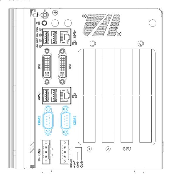
The system provides totally five COM ports for communicating with external devices. These COM ports are implemented using industrial-grade ITE8786 Super IO chip (-40 to 85°C) and provide up to 115200 bps baud rate.
