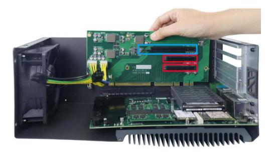
The system has two x8 (indicated in red) and one x16 (indicated in blue) PCI Express slot. The x8 slot is running at Gen3, 4-lanes PCIe signals and can deliver up to 7.9GB/s bandwidth. The x16 slot is running at Gen3, offering 16-lanes PCIe signals and can deliver up to 15.8GB/s bandwidth. The x16 PCIe slot is suitable for both graphics card and I/O card installation.
