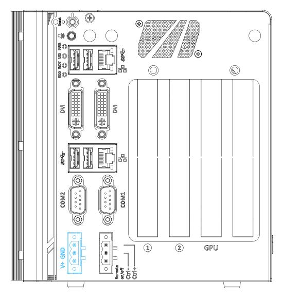
The system accepts 24V DC power input via a 3-pin pluggable terminal block, which is fit for field-use where DC power is usually provided. The screw clamping mechanism on the terminal block offers connection reliability when wiring DC power.
