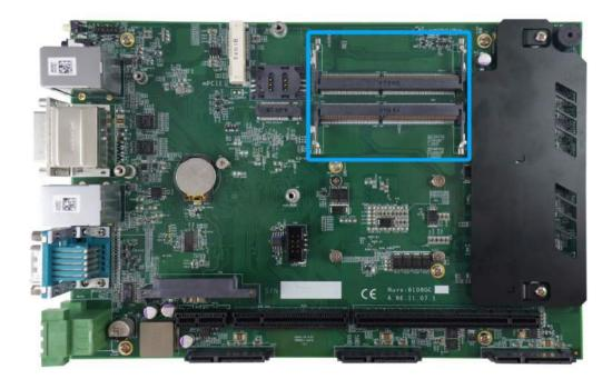
The system motherboard supports two 260-pin SODIMM socket for installing DDR4 memory module up to 32GB. Each slot supports single module DDR4 2133MHz SODIMM up to 16GB capacity.
