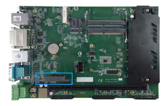
The system features four SATA ports. SATA port No. 1 located near the center of the motherboard via a 22-pin SATA connector. You can directly mount a 2.5" HDD/SSD to this port using the bracket that came with the system. For installing procedures, please refer to "Installing HDD/ SSD to SATA Port 1".
