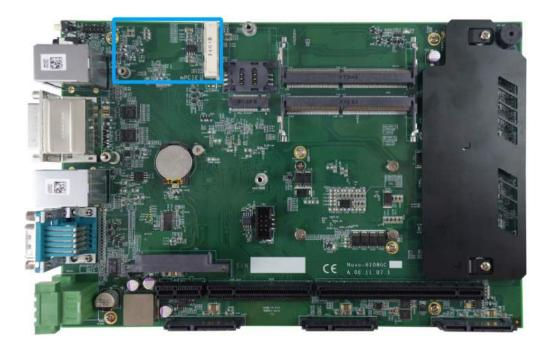
The system has a mini-PCIe slot to accommodate solid-state storage device (SSD) or wireless LAN module. Using SSD offers extreme reliability for harsh environments with intense vibration/shock. The system recognizes mini-PCIe SSD as a native storage device so you may install any operating system on the mini-PCIe SSD module, such as Windows 7, Windows 8, Windows 10, Linux and etc.
