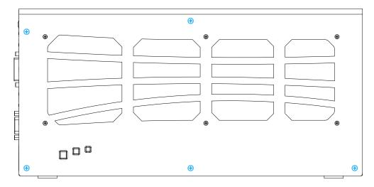
4. Unscrew the two screws on the system ventilation fan panel shown below.
