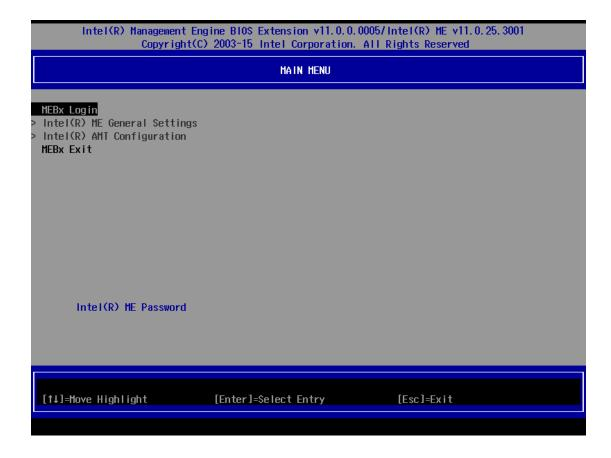
Highlight MEBx Login and press Enter, a prompt will appear asking for password. The default password is "admin". For further MEBx configuration details, please refer to <a href="Intel® MEBX User Guide">Intel® MEBX User Guide</a>.
