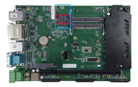
The system has a M.2 (indicated in blue) slot that works in cooperation with a SIM slot (indicated in red). By installing a M.2 module, you can install a 3G/4G module with a SIM card for internet access via your service provider's 3G/4G network.
