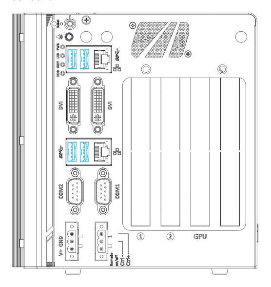
The system's USB 3.0 (SuperSpeed USB) ports are implemented by native xHCI (eXtensible Host Controller Interface) controller and are backward compatible with USB 2.0, USB 1.1 and USB 1.0 devices. Legacy USB is also supported so you can use USB keyboard/mouse in DOS environment
