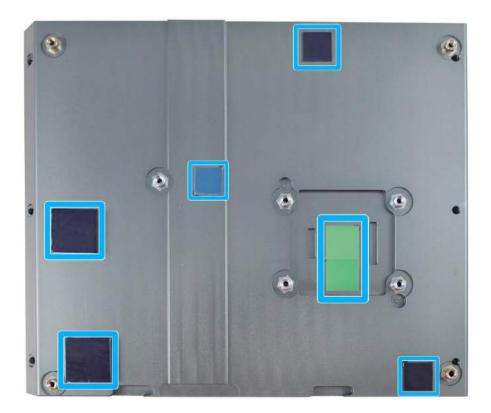
6. With the five motherboard standoffs aligned, gently lower the motherboard onto the heatsink.
