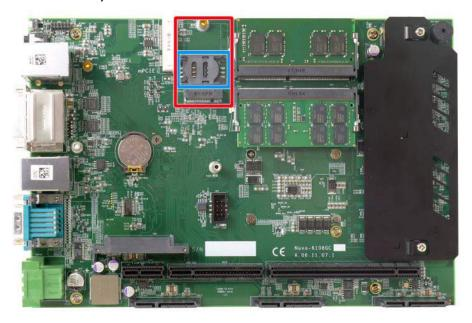
The system has a M.2 slot (indicated in red) coupled with SIM socket (indicated in blue) for installing 3G/4G module. For installation, please refer to the following instructions.
