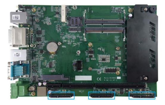
The system has a total of four SATA ports. In addition to SATA port No. 1 mentioned in the previous section, from left to right, SATA port No. 2, 3 and 4 are located at the bottom of the motherboard via 22-pin SATA connectors. The hard drive/ SSD must be secured onto the hard drive tray that came with the system. For installation procedures, please refer to <a href="Installing HDD/SSD">Installing HDD/SSD</a> to SATA Ports 2/3/4.
