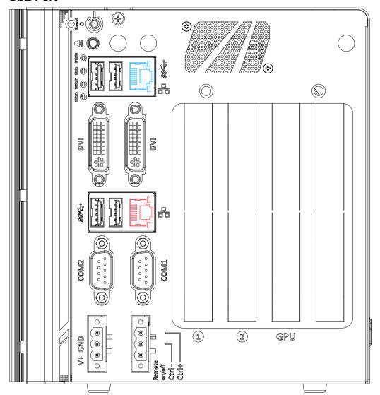
The system offers 2 GbE ports on its I/O panel. The GbE ports are marked in blue/
