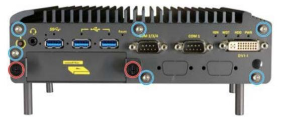
4. Remove the screw indicated on the rear I/O panel and separate it from the enclosure.
