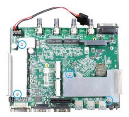
2. Slide bottom U-shape panel to align with the heatsink.
