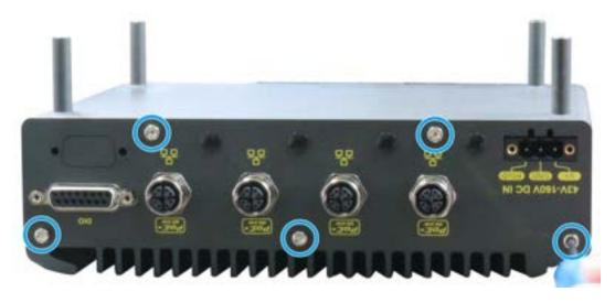
5. Use a small Phillips screwdriver to loosen the screws for 3-pin connector, and unplug it.
