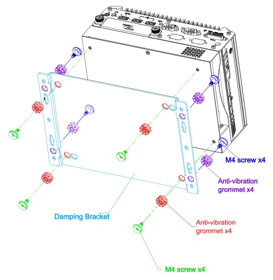
Referring to the illustration shown above, insert four anti-vibration grommets into
