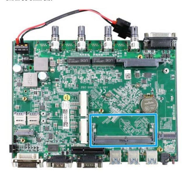
The system motherboard supports a SODIMM socket for installing a DDR4-3200 memory module up to 32GB capacity.
