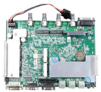
3. Remove the heatsink to access the M.2 slot
