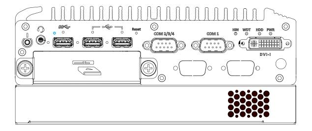
The CMOS Reset button is used to manually reset the motherboard BIOS in case of system halt or malfunction. To avoid unexpected operation, it is purposely placed behind the panel. To reset, please use the tip of a pen, press and hold for at least 5 seconds to reset the BIOS.
