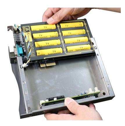
Remove the new supercapacitor UPS module out of the delivered enclosure/ static bag.
