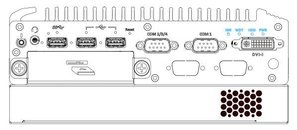
There are four LED indicators on the I/O panel: PWR, WDT, HDD and IGN. The descriptions of these LEDs are listed in the following table.
