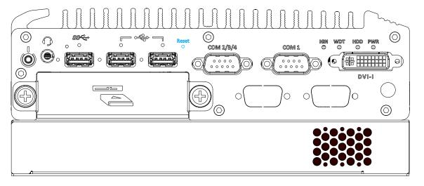
The reset button can be used to manually reset the system in case of abnormal condition. To avoid unexpected operation, the reset button is hidden behind the front panel. You need to use a pin-like object to push the reset button.
