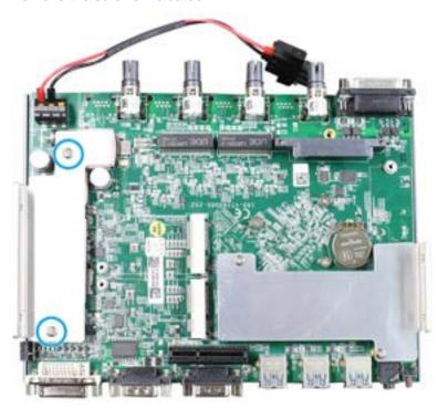
3. Remove the heatsink to access the M.2 3042/ 3052 B key and SIM card slots.
