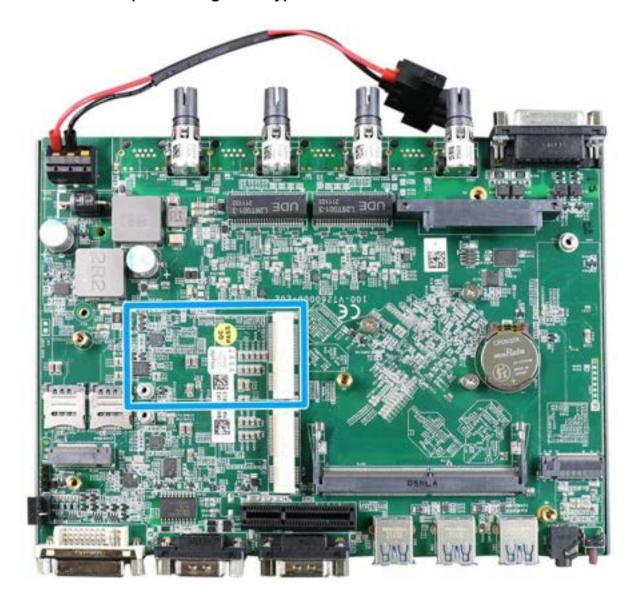
There is a full-size USB2.0 signal only mini-PCIe socket for better compatibility with off-the-shelf mini-PCIe wireless modules. For customers who want to install a mini-PCIe wireless module, please take advantage of the mini-PCIe socket and the antenna openings on the panels.
