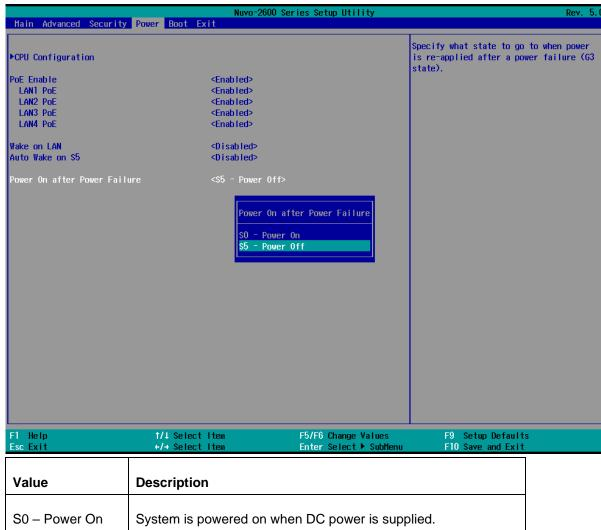
S5 - Power Off System is kept in off state when DC power is supplied.
