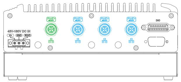
The system offers four PoE+ GbE ports via M12 X-coded connectors on the front panel. The ports are implemented using Intel® I210 controller and the port indicated in **green** supports Wake-on-LAN.
