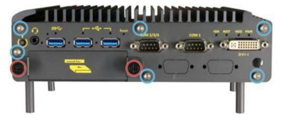
6. Secure the screws (indicated in blue) on the M12 connector panel.
