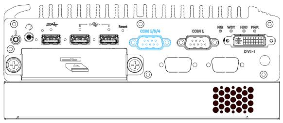
Implemented using industrial-grade ITE8786 Super IO chip (-40 to 85°C) and provide up to 921600 bps baud rate, the second D-Sub male connector (COM2/ 3/ 4) can be configured in BIOS as single RS-422/ 485 port (COM2) or three 3-wire RS-232 ports (COM2/COM3/COM4). Please refer to COM2/ 3/ 4 Port Configuration for configuring operation mode. An optional 1-to-3 Y-cable is available to connect three RS-232 devices.
