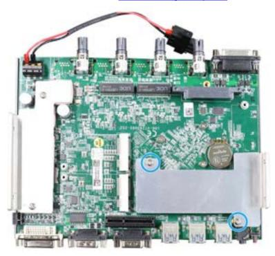
2. Remove the heatsink to locate the SODIMM memory module slot on the motherboard.
