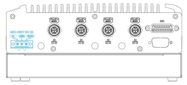
The system accepts a wide range of DC power input from 43V to 160V via a 3-pin pluggable terminal block, which is fit for field usage where DC power is usually provided. The screw clamping mechanism on the terminal block offers connection reliability when wiring DC power.
