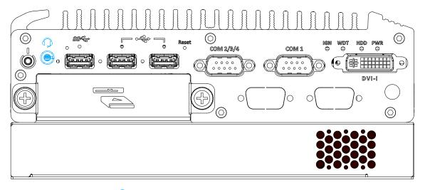
There is a female 4-pole audio jack for headphone (speaker) output and microphone input. To utilize the audio function in Windows, you need to install corresponding drivers. Please refer to the section, <u>Driver Installation</u>.
