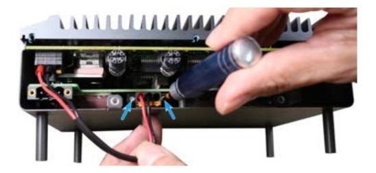
Release screws on the 3-pin connector
