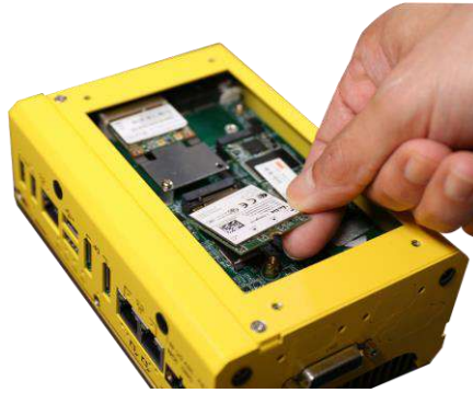
Insert on a 45 degree angle
