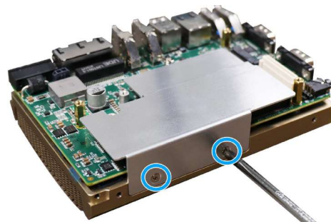
Secure the module heatsink
