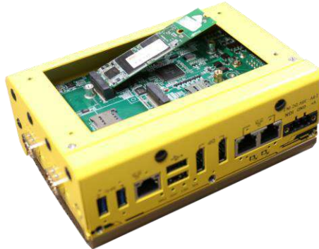
Insert on a 45 degree angle
