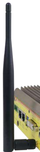
Secure antenna body on enclosure
