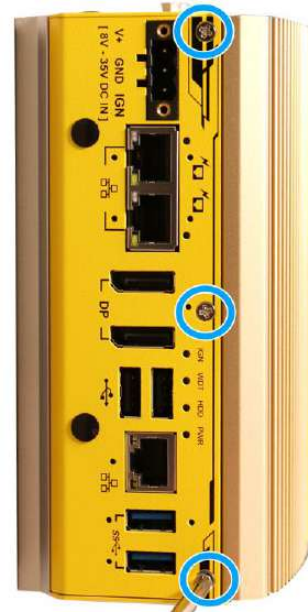
Screws on front panel
