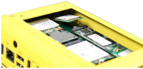
Insert on a 45 degree angle
