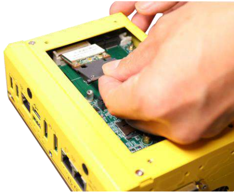
Insert on a 45 degree angle
