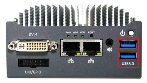
There are totally three USB 3.0 ports and one USB 2.0 port on POC-200 series. Two of three USB 3.0 ports are located on the front panel. They are implemented via a Renasas uPD720202 USB3 host controller. By BIOS default, these USB ports are operated in xHCI (eXtensible Host Control Interface) mode and are compatible to USB 3.0, USB 2.0, USB 1.1 and USB 1.0 devices. Legacy USB support on these ports is provided only when "xHCI Mode" option in BIOS is configured as "Smart Auto".
