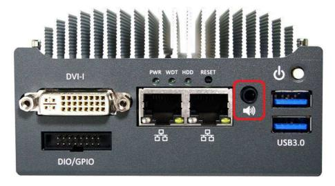
POC-200 series provides speaker-out function using Intel® High Definition Audio (built-in in ICH8-M) and Realtek ALC262 codec. An audio jack is located on the front panel. To utilize
