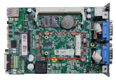
Tilt the mini-PCle WIFI module and insert it to the mini-PCle port. And fix the WIFI module with two M2.5 P-head screws.
