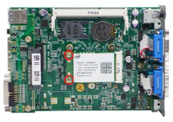
3. Attach the IPEX-to-SMA cable to the WIFI module and fix the SMA connector (on the IPEX-to-SMA cable) to back panel.
