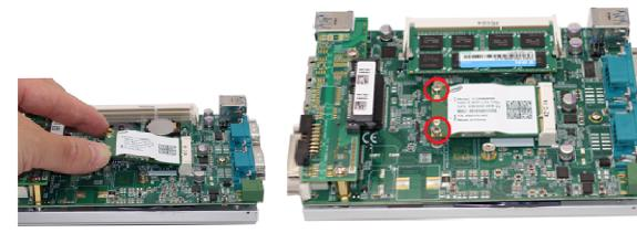
3. Attach the IPEX connector of the IPEX-to-SMA cable to the WIFI module.
