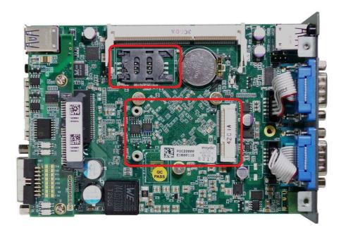
POC-200 series provides an on-board Mini PCI Express socket with SIM card support. There are plenty of off-the-shelf mini-PCIe modules with versatile capabilities. By installing a mini-PCIe module, your system can have expanded features such as WIFI, 3G, GPS, RAID and etc. In addition, the SIM card support makes it possible to connect your system to Internet in wide territory through telecom operator's GPRS/3G network.
