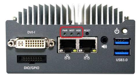
There are three LED indicators on the front panel: PWR, WDT and HDD. The descriptions of these three LED are listed in the following table.
