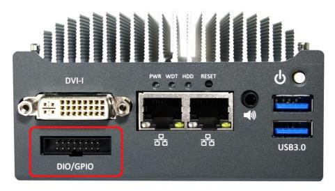
POC-200 integrates 2500Vrms isolated DIO function for extending application range. This feature provides 4 channels of isolated digital input and 4 channels of isolated digital output via a 16-pin box-header connector. The following table describes the pin definition of isolated DIO connector.
