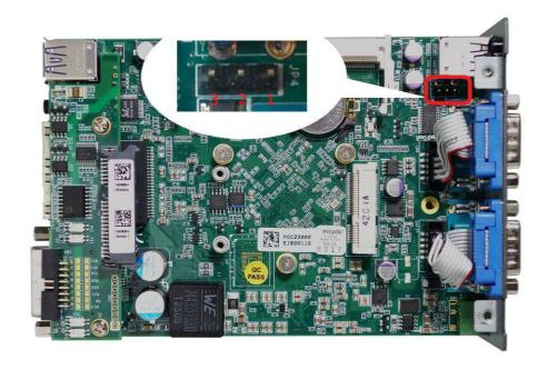
The remote on/off control function allows users to turn on or turn off the system remotely by connecting an external switch. This function is provided via a 1x3 pins, 2.0mm pitch pin header.
