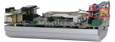
4. Carefully push back the case and fix the chassis/HDD assembly using four M4 F-head screws.
