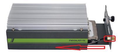
6. Attach the WIFI antenna to the SMA connector.
