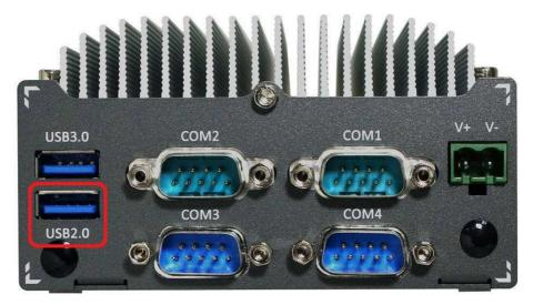
In addition to three USB 3.0 ports, POC-200 series provides another USB 2.0 port on its back panel. By BIOS default, these USB 2.0 ports are operated in EHCI (Enhanced Host Control Interface) mode and are compatible with USB 2.0, USB 1.1 and USB 1.0 devices. Legacy USB support is provided so you can use USB keyboard/mouse in DOS environment.
