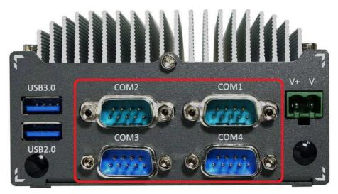
POC-200 and POC-210 provide four COM ports via four 9-pin D-Sub male connectors on the back panel for communicating with external devices. They are implemented using industrial-grade ITE8783 Super IO chip (-40 to 85°C) and provide up to 115200 bps baud rate.
