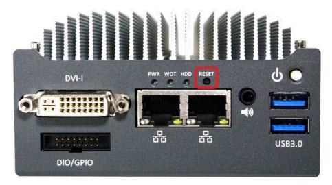
The reset button is used to manually reset the system in case of any abnormal condition. To avoid unexpected operation, the reset button is hidden behind the front panel. You need to use a pin-like object to push the reset button.
