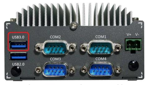
There are totally three USB 3.0 ports and one USB 2.0 port on POC-200 series. One of three USB 3.0 ports is located on the back panel. This USB 3.0 port is implemented via native xHCI controller inside Bay Trail SoC. By BIOS default, this USB port is operated in xHCI (eXtensible Host Control Interface) mode and is compatible to USB 3.0, USB 2.0, USB 1.1 and USB 1.0 devices.
