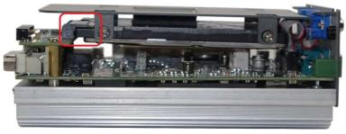
5. Carefully push back the case and fix the chassis assembly using four M4 F-head screws.
