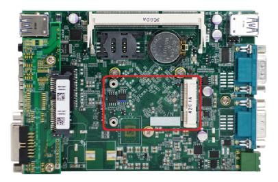
2. Tilt the mini-PCle WIFI module and insert it to the mini-PCle port. And fix the WIFI module with two M2.5 P-head screws.
