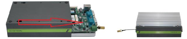
5. Fix the SMA connector of the IPEX-to-SMA cable to back panel.
