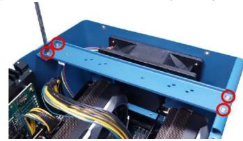
Secure the GPU bracket onto the chassis GPU bracket by securing the two screws for each GPU bracket.
