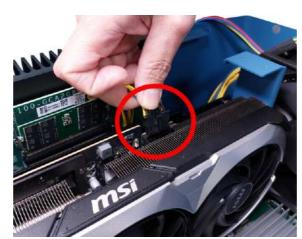
1 If you are installing dual GPUs, install the cross bar that is positioned at the back of the GPU bracket.
