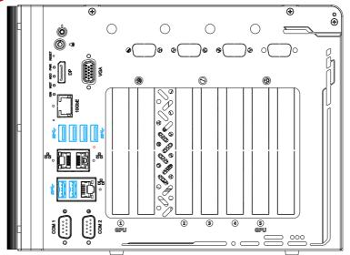
The system's USB 3.2 Gen2x1ports (10Gbps) are implemented via native xHCI (eXtensible Host Controller Interface) controller and are backward compatible with USB3.2 Gen.1, USB 2.0, USB 1.1 and USB 1.0 devices. UFEI USB is also supported so you can use USB keyboard/mouse in UEFI shell environment. Indicated in **red** is a screw-lock hole for the corresponding USB port.
