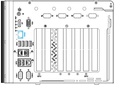
The optional high-speed data transmission 10G Ethernet port is backward compatible with 5GBASE-T and 2.5GBASE-T to work with NBASE-T industrial cameras. Indicated in **red**is a screw-lock hole for the corresponding Ethernet port.
