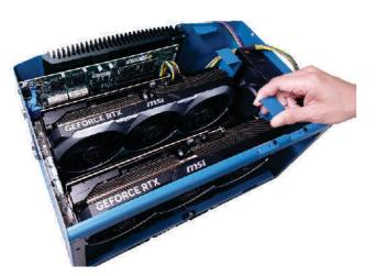
Plug in the power cable(s) onto the graphics card(s).
