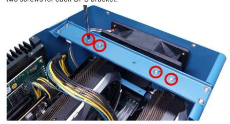
Secure the screws indicated on the I/O panel to complete the graphics card installation process.
