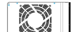
d Remove the screws indicated at the rear of the enclosure.
