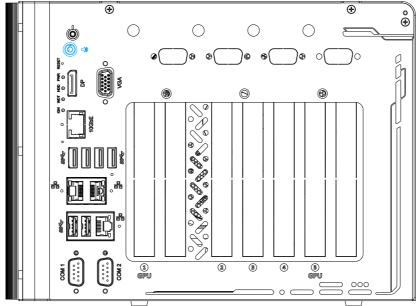
The system audio function uses high definition audio. There is a female 4-pole audio jack for headphone (speaker) output and microphone input. To utilize the audio function in Windows, you need to install corresponding drivers for both Intel chipset and audio device drivers.
