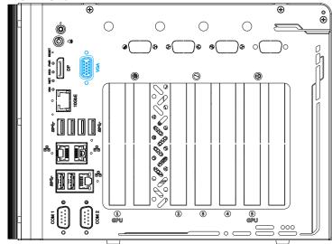
VGA connector is the most common video display connection. The VGA output supports up to 1920x1200@60Hz resolution. The system supports dual independent display outputs by connecting display devices to VGA, and DisplayPort. To support multiple display outputs and achieve best VGA output resolution in Windows, you need to install corresponding graphics drivers.
