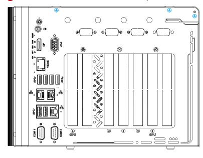
Remove the screws indicated on the side panel.
