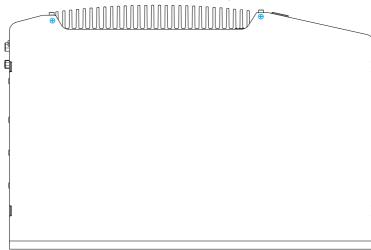
Remove the GPU chassis bracket by removing the four screws.
