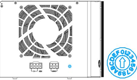
To have ignition power control for in-vehicle usage, you need to supply IGN signal to the system. The IGN input is located on the 4-pin pluggable terminal block (shared with DC power input). Below is the typical wiring configuration for in-vehicle applications.
