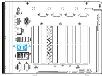
The system offers 2.5GbE ports on its I/O panel. Marked in red are screw-lock mechanism for rugged connectivity. Each port has dedicated PCI Express link for maximum performance. When an Ethernet connection is established, the LED indicators on the RJ45 connector represents the following connection statuses:
