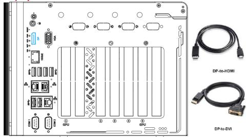
The DisplayPort (DP) output is a digital display interface that mainly connect video source and carry audio to a display device. When connecting a DP, it can deliver up to 4K UHD (4096 x 2304) in resolution. The system is designed to support passive DP adapter/ cable. You can connect to other display devices using DP-to-HDMI cable or DP-to-DVI cable.
