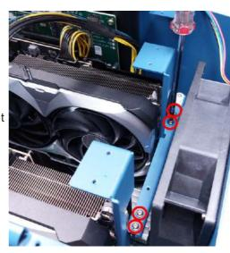
Place the L-shaped panel back onto the enclosure..
