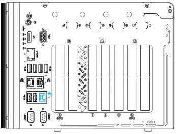
The systemhas a GbE port and supports Wake-on-LAN. It is implemented with Intel® I219-LM controller with a dedicated PCI Express link for maximum performance. The LED indicators on the RJ45 connector represents the following connection statuses:
