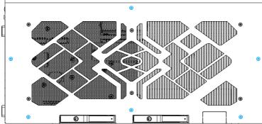
© Remove the screws indicated on top of the enclosure.
