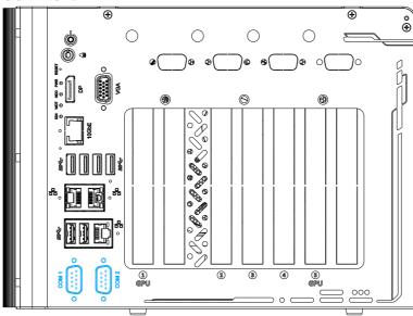
Providing up to 115200 bps baud rate, COM1 and COM2 are software-configurable RS-232/422/485 ports. The operation mode can be set in BIOS setup utility. The following table describes the pin definition of COM ports.
