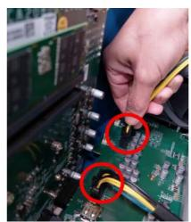
slot furthest away from the motherboard if you are only installing one graphics card.
