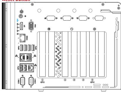
The reset button is used to manually reset the system in case of system halt or malfunction. To avoid unexpected reset, the button is purposely placed behind the panel. To reset, please use a pin-like object (eg. tip of a pen) to access the reset button
