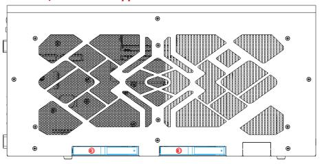
The system has two external 2.5" HDD/ SSD hot-swappable slots. Designed for easy access, the HDD/ SSD slots are secured by a lock (indicated in red) and it supports RAID modes 0/1 configurations.
