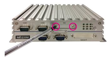
2. Remove the tray of the M.2 socket.
