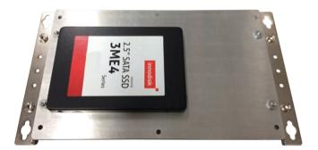
2. While supporting the SATA drive, turn the cover to the other side. This will be the outer side of the cover. Use the provided screws to secure the drive in place.
