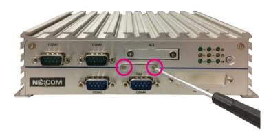
2. Insert the SIM card into the slot.
