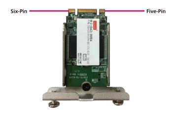
6. Insert the M.2 module and fasten the cover.
