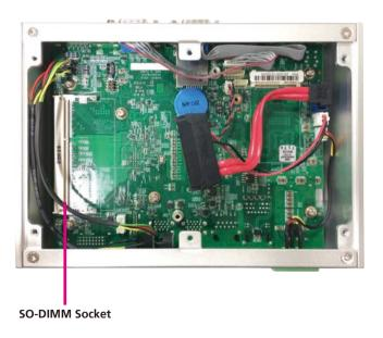
2. Insert the module into the socket at an approximately 30 degrees angle. The ejector tabs at the ends of the socket will automatically snap into the locked position to hold the module in place.
