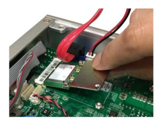
4. Push the module down and secure it with a screw.
