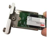
4. Secure the module with a screw.
