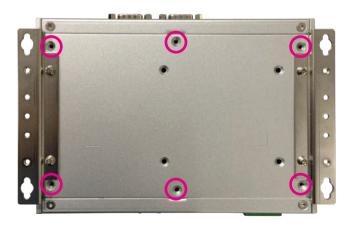
2. Remove the 6 screws on the bottom side of the chassis cover.
