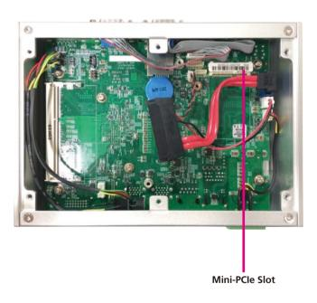
2. Install the mini-PCle bracket to the mini-PCle module.
