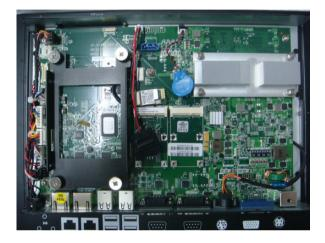
8. Attach one end of the RF cable onto the module.
