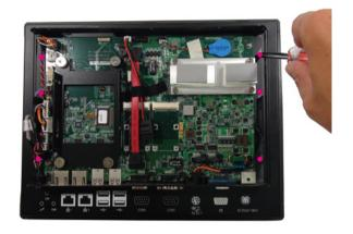
3. Gently lift the motherboard support plate upwards and locate the SODIMM socket underneath.
