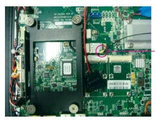
Attach RF cable to the module
