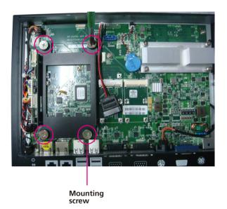
4. Remove the drive bay and locate the Bluetooth connector and mounting hole on the mainboard.
