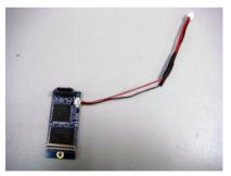
6. Install the module to the SATA port via the connector at the solder side of the module and then secure the module using the mounting screw you removed in step 2.
