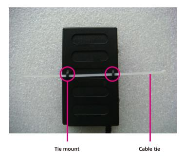
5. Wrap the power adapter cable, then secure the cable firmly by tying the cable tie.
