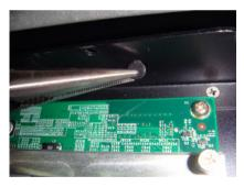
6. Insert the antenna jack end of the cable through the antenna hole.
