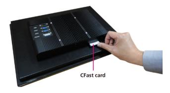
4. Push the CFast card to remove the CFast card.
