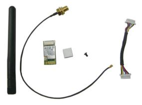
1. Remove the sticker on one side of the square rubber pad, then place that side on the back of the Bluetooth module.
