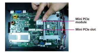
2. Secure the module with mounting screws.
