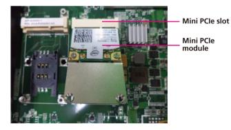
2. Secure the module with mounting screws.
