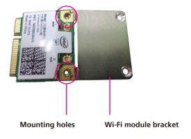
2. Tighten screws onto the mounting holes to secure the bracket.
