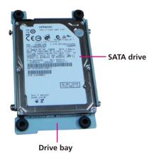
5. Align the mounting holes that are on the sides of the SATA drive with the mounting holes on the drive bay and then use the provided mounting screws to secure the drive in place.
