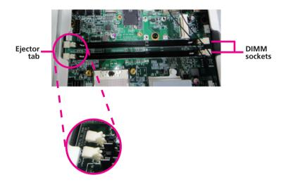
2. Note how the module is keyed to the socket. Grasping the module by its edges, align the module with the socket so that the "notch" on the module is aligned with the "key" on the socket. The key ensures the module can be plugged into the socket in only one direction.
