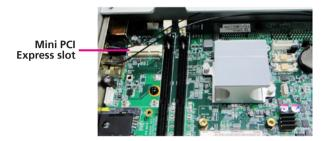
2. Insert the wireless LAN module into the Mini PCI Express slot at a 45 degrees angle until the gold-plated connector on the edge of the module completely disappears inside the slot.
