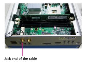
6. Connect an external antenna to the antenna jack.
