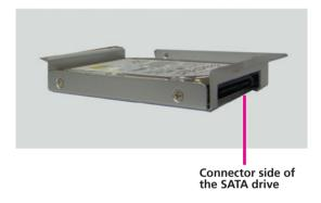
6. Connect the SATA data cable and SATA power cable to the connectors on the SATA drive.
