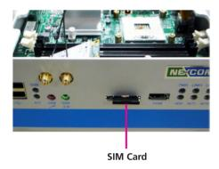
2. To take out the SIM card, push the yellow button using a pointed object.
