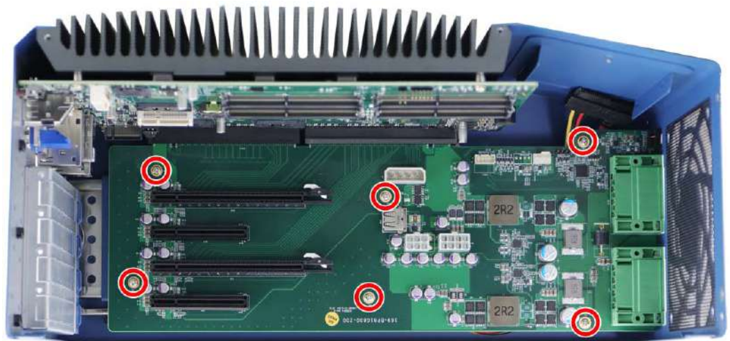
Remove screws to separate the extension board from the motherboard
