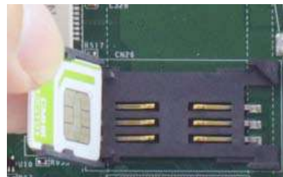
Insert Mini-SIM card with pins facing up
