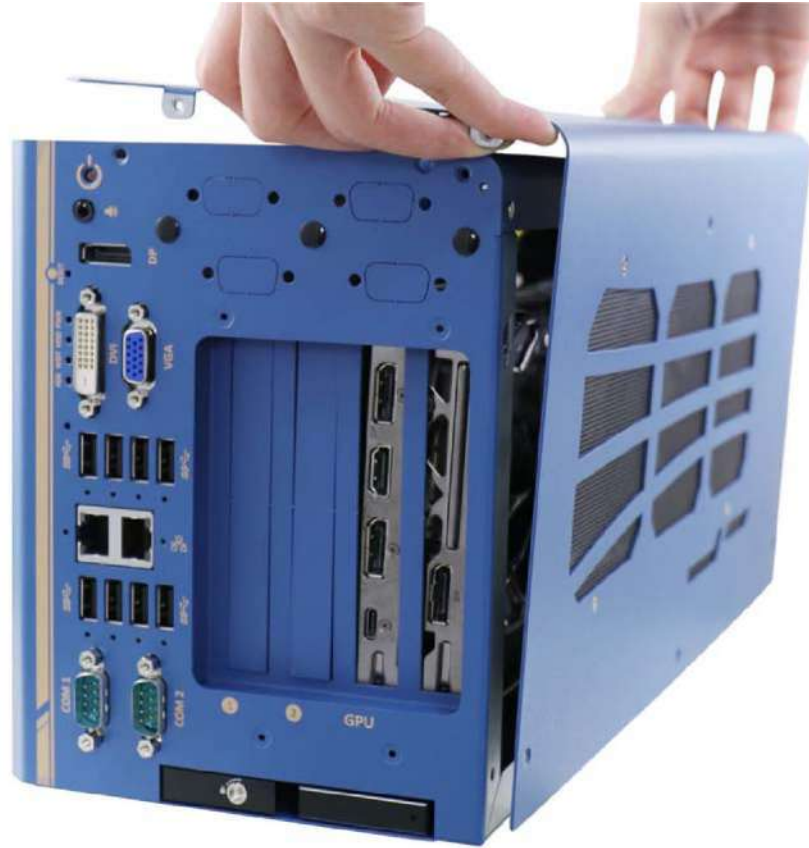
Place L-shape side panel onto the enclosure
