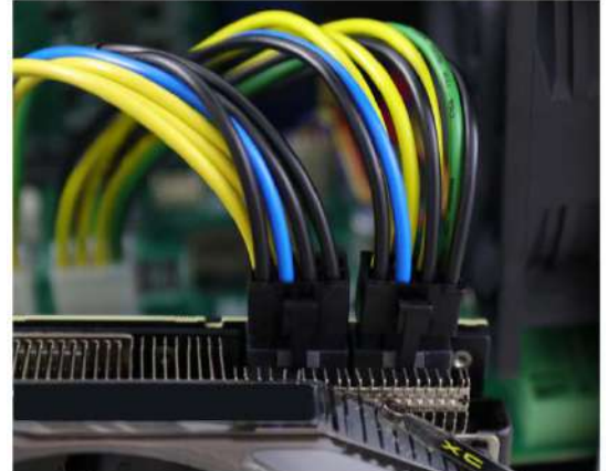
6 or 8/ 8-pin power connector on graphics card
