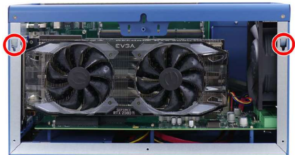
Slide-and-lock into the indicate hinges
