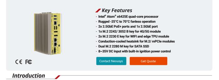
POC-451VTC is an ultra-compact in-vehicle computer with E-Mark certificate for in-vehicle applications, such as mobile gateway, mobile surveillance and passenger information system. It leverages the latest Intel<sup>®</sup> Elkhart Lake Atom<sup>®</sup> x6425E CPU, delivering 1.8x and 2x performance improvement for the CPU and GPU respectively, compared to the previous generation.
