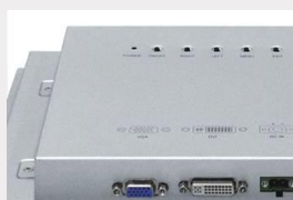
OSD control buttons on the rear panel
