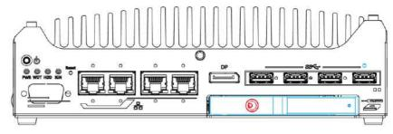
The system features an external hot-swappable 2.5" hot-swappable tray that supports a 7mm 2.5" HDD/ SSD. Designed for easy access, the HDD tray is secured by a lock (indicated in red).
