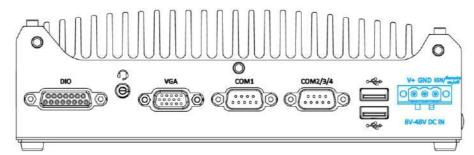
The system accepts a wide range of DC power input from 8 to 48V via a 3-pin pluggable terminal block, which is fit for field usage where DC power is usually provided. The screw clamping mechanism on the terminal block offers connection reliability when wiring DC power.
