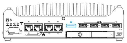
The system has a DisplayPort (DP) output which is a digital display interfaces that mainly connect video source and carry audio to a display device. When connecting a DP, it can deliver up to 4K UHD (4096 x 2304) in resolution. The system is designed to support passive DP adapter/ cable. You can connect to other display devices using DP-to-HDMI cable or DP-to-DVI cable.
