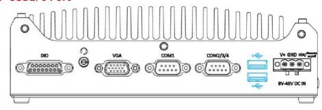
The USB2.0 ports are implemented via native xHCI (eXtensible Host Controller Interface) in the Intel 600 chipset and are backward compatible with USB 1.1 and USB 1.0 devices. UEFI USB support is also provided so you can use USB keyboard/ mouse in UEFI shell environment.
