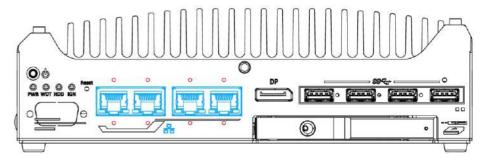
The system offers four 2.5Gb Ethernet ports using Intel® I226 controller, and each port each come with screw-lock mechanism (indicated in red). When plugged in and connected via the Ethernet cable, the LEDs on the RJ45 connector indicate connection status and speed.
