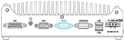
The port provides up to 921600 bps baud rate, it is a software-configurable RS-232/422/485 port via 9-pin D-Sub male connector. The operation mode, slew rate and termination of COM1 can be set in BIOS setup utility. The following table describes the pin definition of COM ports.
