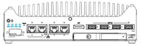
There are four LED indicators on the I/O panel: PWR (power), WDT (Watchdog timer), HDD (hard disk drive), IGN (ignition power control, an optional feature). The descriptions of these four LED are listed in the following table.
