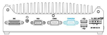
The port provides up to 921600 bps baud rate, it can be configured in the BIOS as single RS-422/485 port (COM2) or three 3-wire RS-232 ports (COM2/3/4). An optional 1-to-3 Y-cable is available to connect three RS-232 devices.
