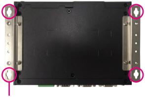
Fasten screws to mount the system to the wall
