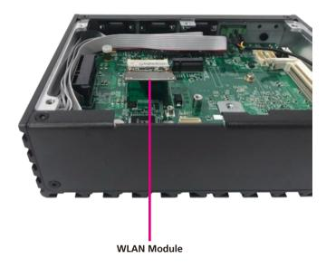
4. Push the module down and secure it with a screw.
