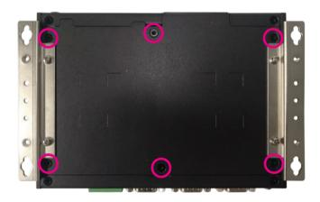
2. Remove the six mounting screws from the bottom cover.
