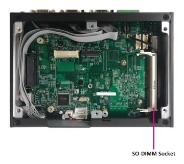
2. Insert the module into the socket at an approximately 30-degree angle. The ejector tabs at the ends of the socket will automatically snap into the locked position to hold the module in place.
