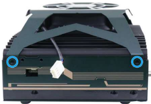
Secure the two screws
