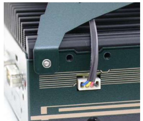
Plug in the 4-pin power connector
