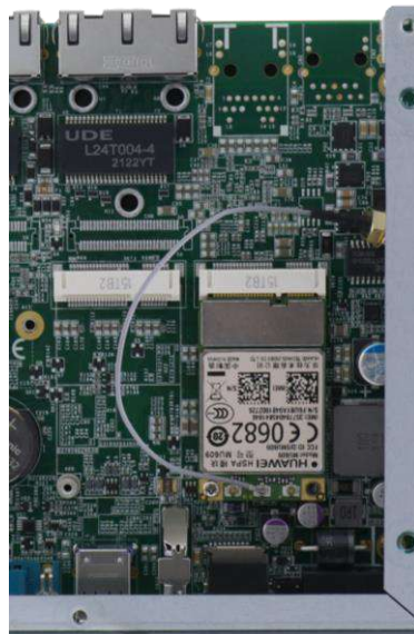
Clip on the IPEX-to-SMA cable
