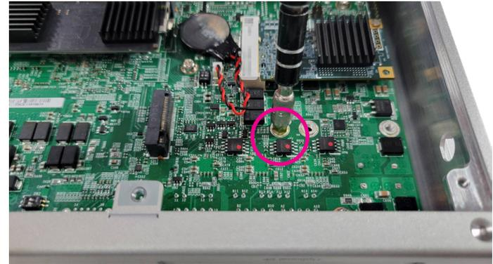
5. Insert the M.2 module into the M.2 slot at an 45-degree until the gold-plated connectors on the edge of the module insert completely.
