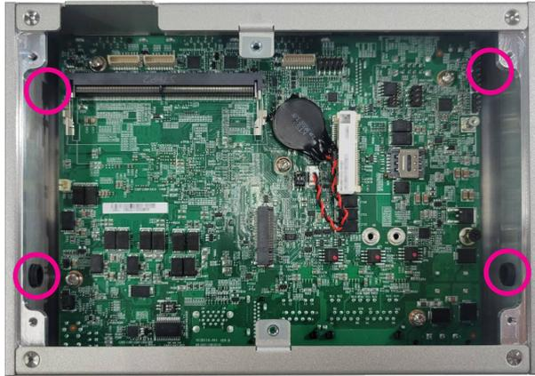
2. Remove the antenna hole plug(s).
