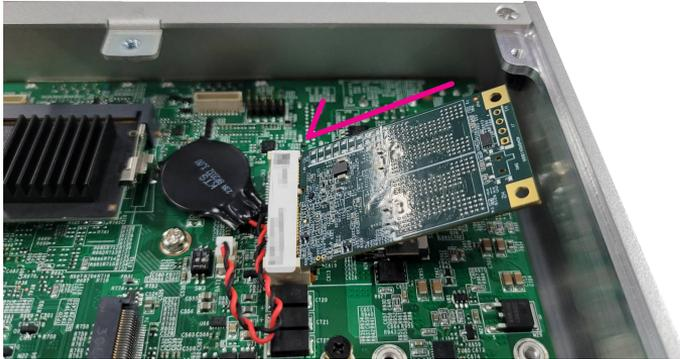
4. Push the module down and secure it with a screw.
