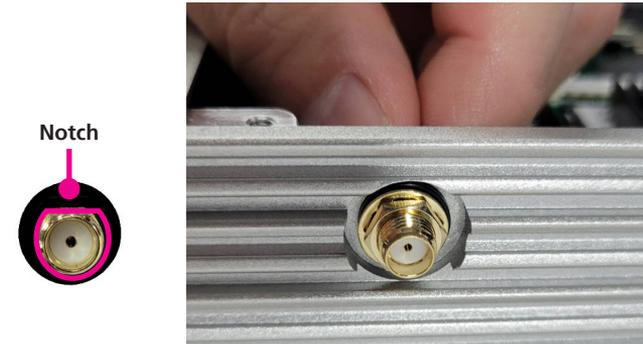
5. Follow the position shown below to install the other antenna washer and antenna components.
