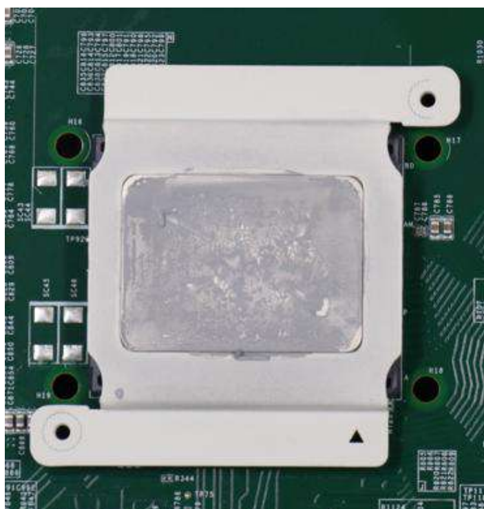
CPU retention bracket (holder)
