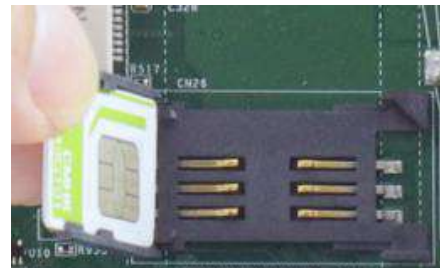
Insert SIM card with pins facing up
