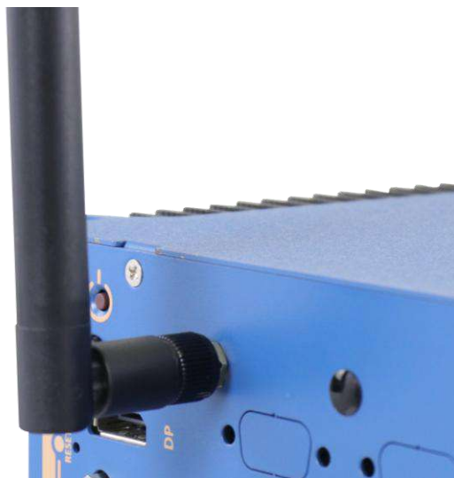
Clip on IPEX-to-SMA cable
