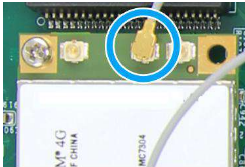
Clip on IPEX-to-SMA cable
