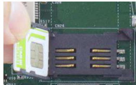
Insert SIM card with pins facing up
