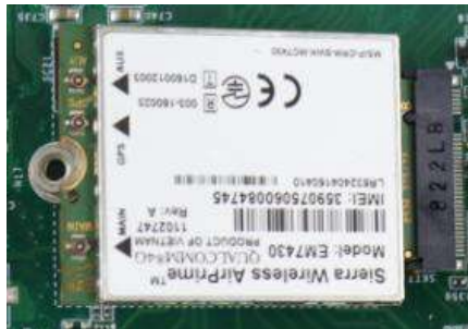
Insert on 45 degree angle
