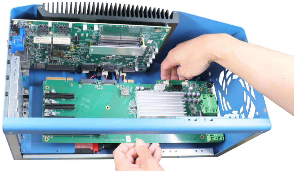
Disengage the daughterboard from the motherboard
