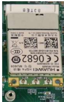
Insert on 45 degree angle
