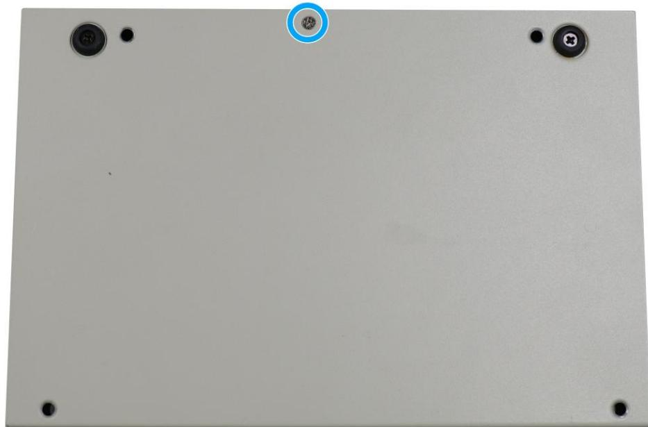
7. Gently lower the Cassette module back onto the system enclosure and secure the module onto the system enclosure by securing the following screws.
