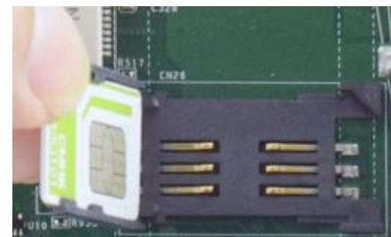
Insert Mini-SIM card with pins
