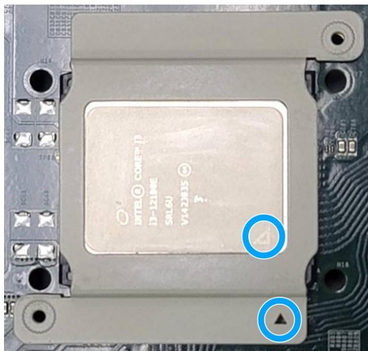
6. Turn the motherboard around while holding the CPU retention bracket in-place, and secure the bracket by tightening two M3 P-head screws on the other side of the motherboard.
