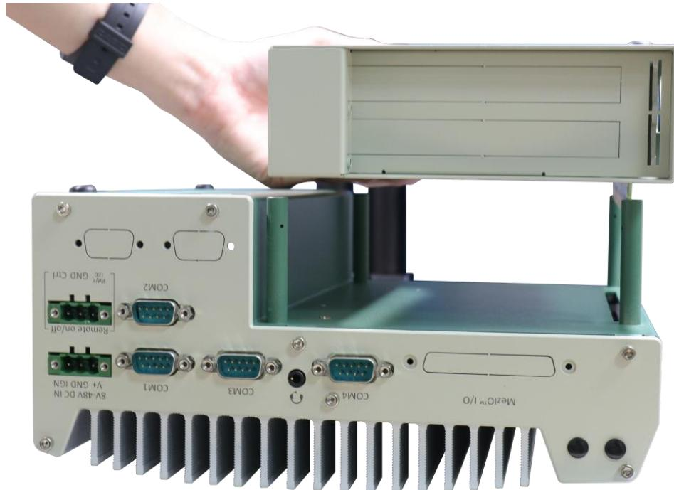
3. On the front I/O panel, remove the hexa-screws indicated below.
