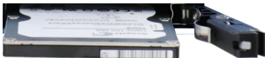
3. Push the handle into the 2.5" slot until it snaps into position. A key is provided (in accessory box) to lock the external slot.
