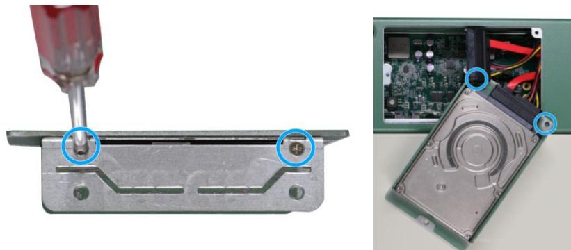
2 screws on each side per HDD/ SSD
