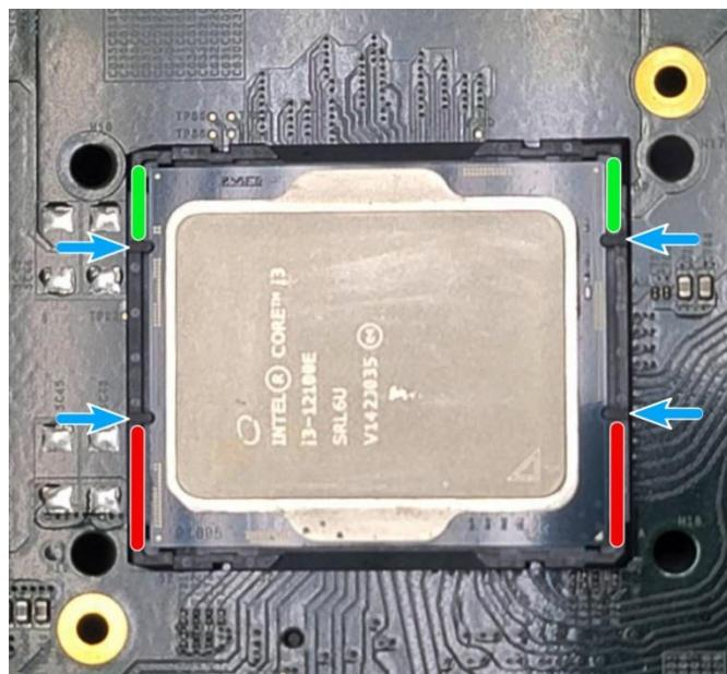
8. Make sure all thermal pad residues have been cleaned on both sides of the retention bracket. Place the CPU retention bracket (holder) on top of the CPU and hold it in place. Make sure the indicator triangle engraved on the CPU's integrated heat spreader (HIS) and the triangle indicator on the retention bracket are positioned in the same corner (indicated by **blue circles**).
