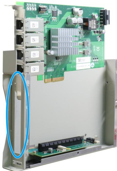
**Remove bezel cover and insert the card**
