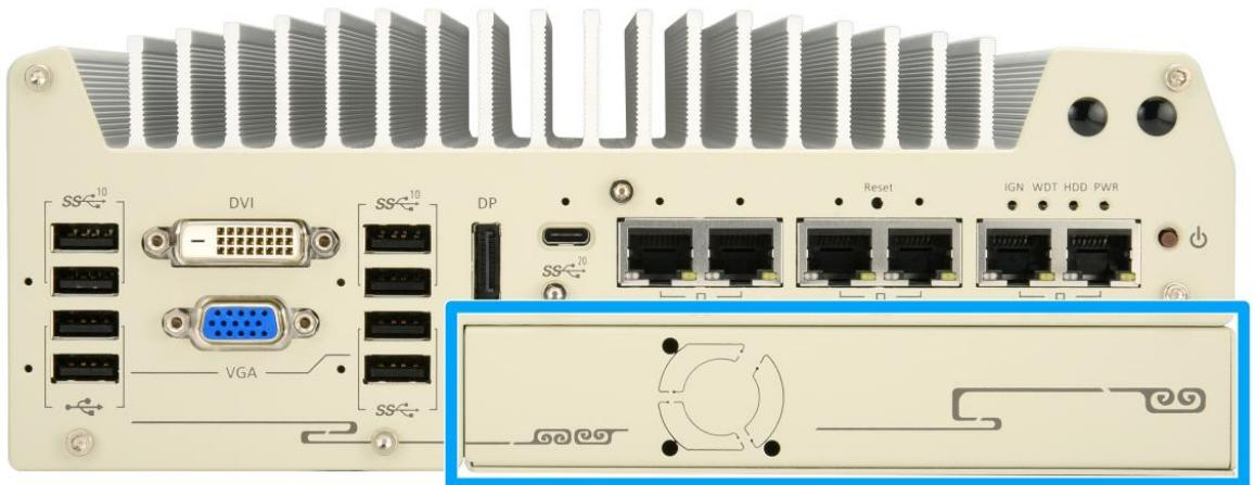
The Cassette module provides a separated compartment to accommodate add-on card(s). It compartmentalizes the heat generated and effectively manages thermal conditions of both the system and add-on card(s). The modular design reduces the complexity of installing and replacing add-on card(s) in the fanless controller. In addition, the mechanical design creates a sealed wind tunnel to bring in cold air and expels hot air via a system fan to offer the system extreme stability and reliability.
