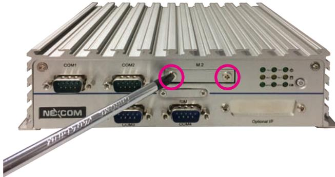
2. Remove the tray of the M.2 socket.
