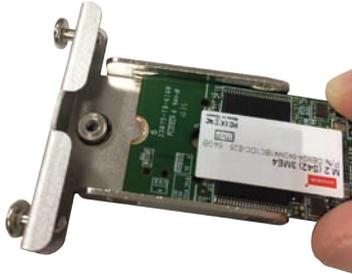
4. Secure the module with a screw.
