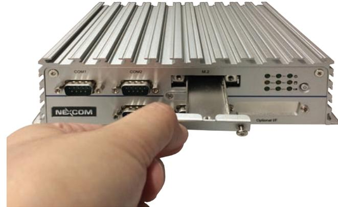
3. Insert the M.2 module into the tray.
