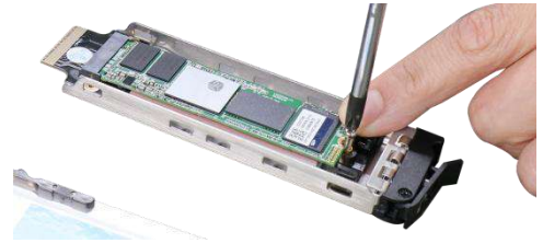
Secure with a screw
