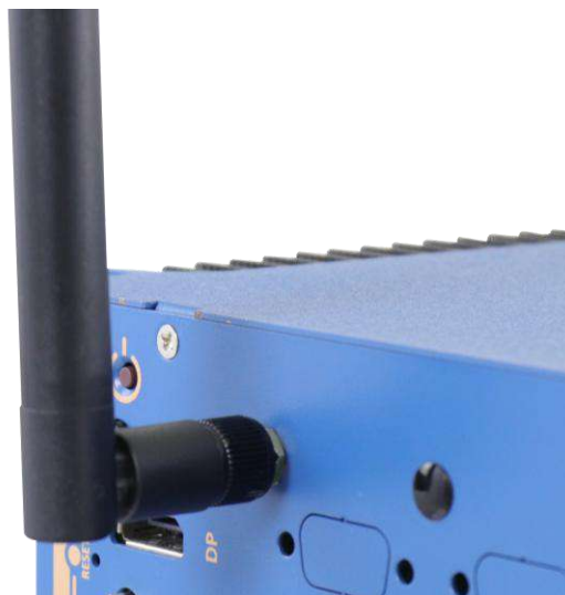
Clip on IPEX-to-SMA cable
