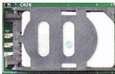
Slide and lift SIM card holder
