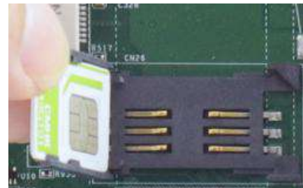
Insert SIM card with pins facing up
