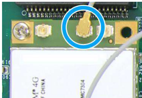
Clip on IPEX-to-SMA cable
