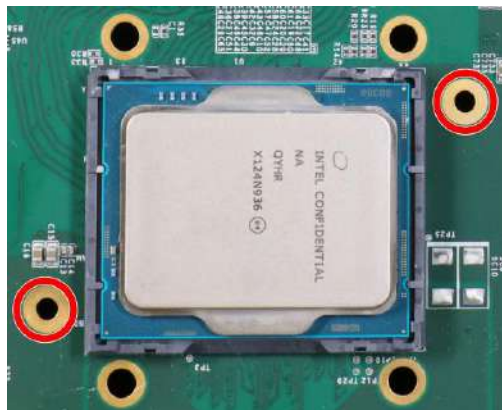
Screw holes for CPU retention bracket
