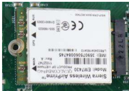
Insert on 45 degree angle
