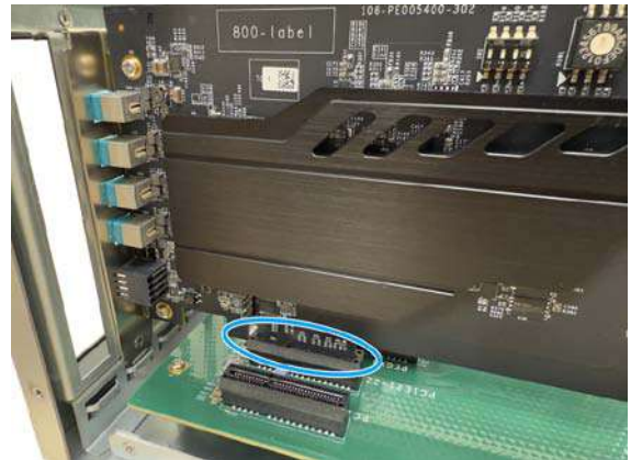
Insert gold fingers into PCIe slot
