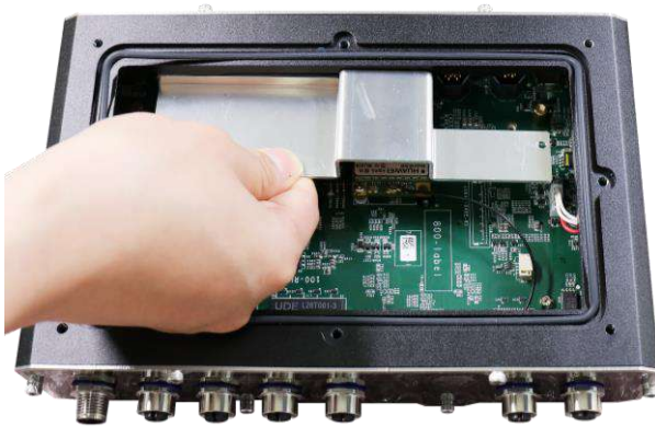
Place heatsink back on the modules
