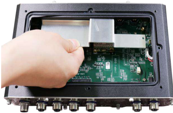
Place heatsink back on the modules
