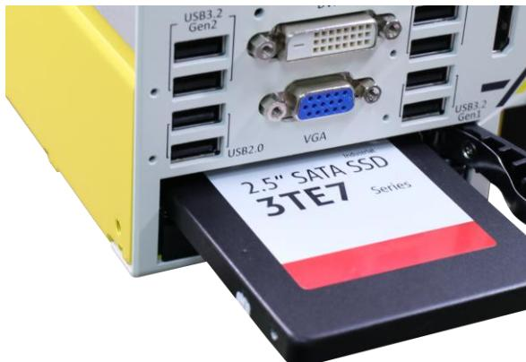
3. Push the lever into the 2.5" slot until it snaps into position. A key is provided (in accessory box) to lock the external slot.
