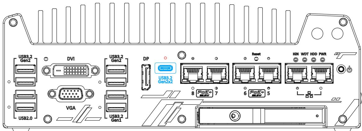
The system's USB 3.2 Gen2x2 type-C port offers up to 20Gbps of data transfer bandwidth, and is implemented via the native xHCI (eXtensible Host Controller Interface) controller. Indicated in red is a screw-lock hole for the corresponding USB port.
