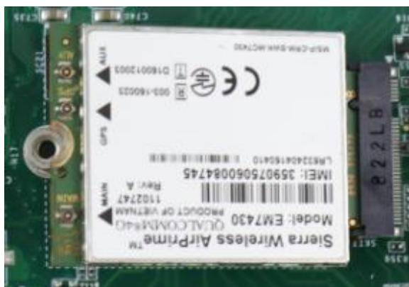
6. Gently press down and secure the module with an M3 P-head screw.
