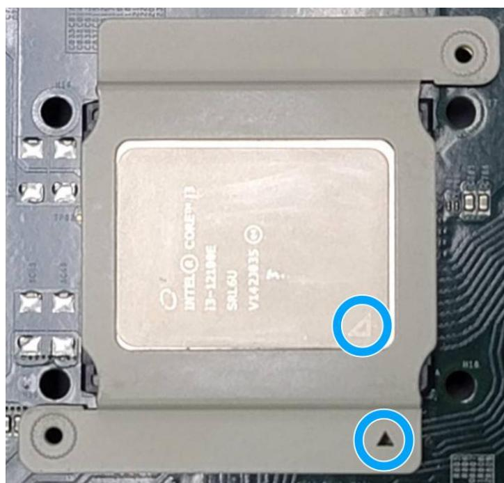
6. Turn the motherboard around and secure the bracket by tightening two M3 P-head screws.
