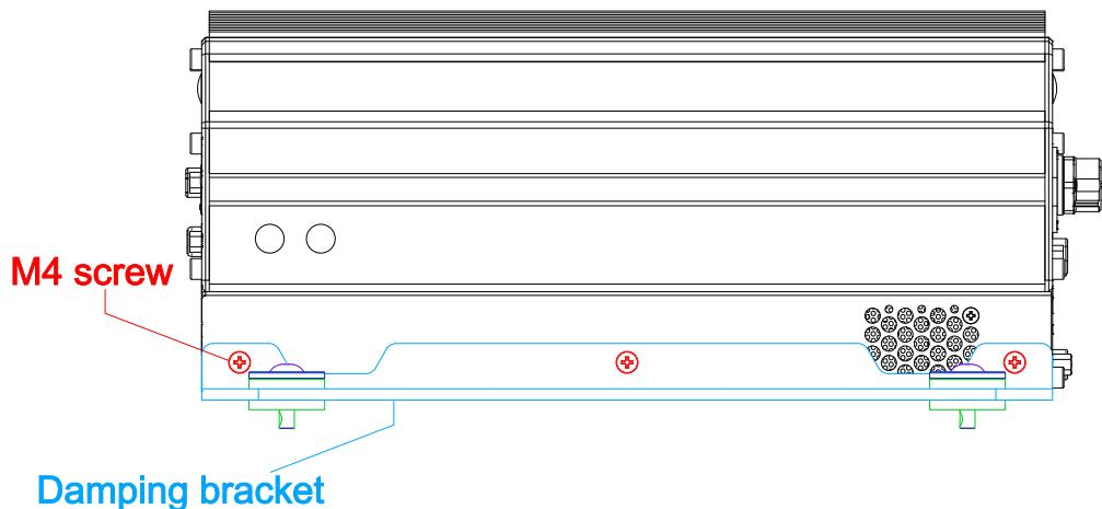
2. Place the system on a flat surface, insert the **sleeves** into the **anti-vibration grommets** and secure it with **M4 screws**.
