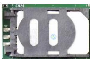
5. Insert the module on a 45 degree angle.
