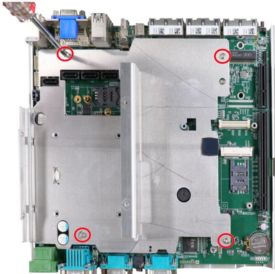
2. To reinstall the system enclosure, place the bottom panel on top of the motherboard while making sure both sides are inserted into the heatsink (indicated in **blue**).
