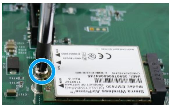
7. For the M.2 module on the MezIO module, the SIM slot is located underneath. Remove the MezIO™ module by removing the screws indicated, and gently lift to separate the module from the motherboard.
