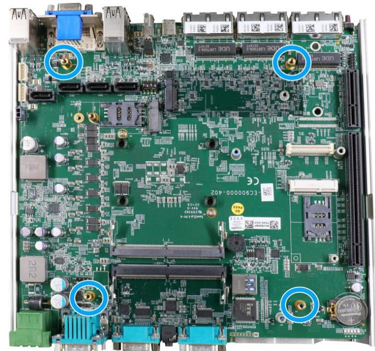
**Secure motherboard with four screws**
