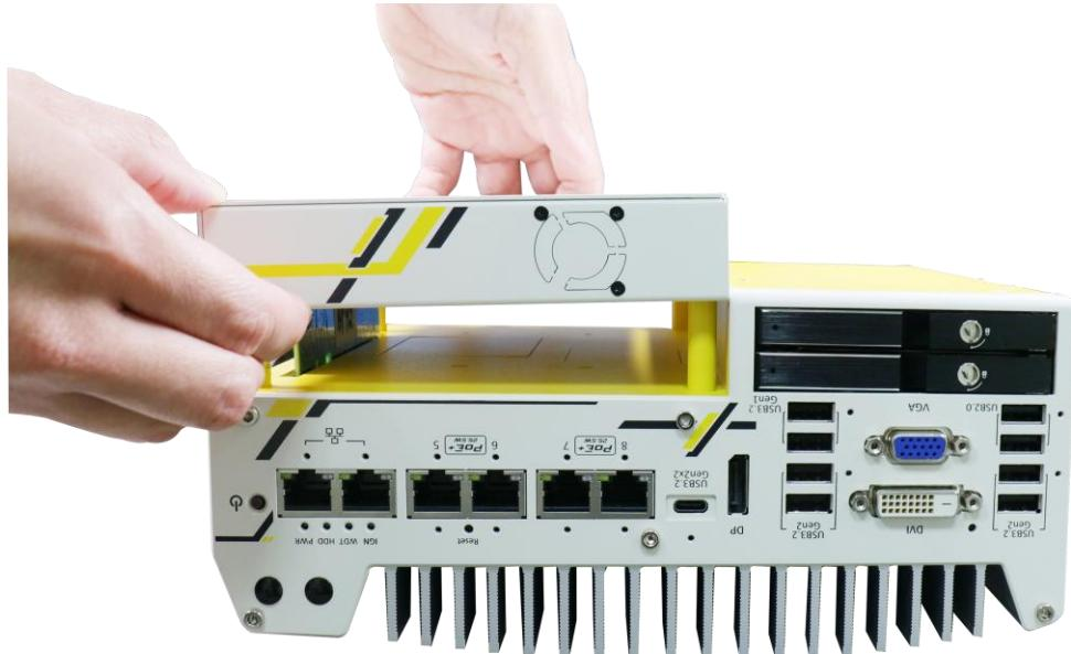
3. On the front I/O panel, remove the screws indicated below, and remove the front panel.
