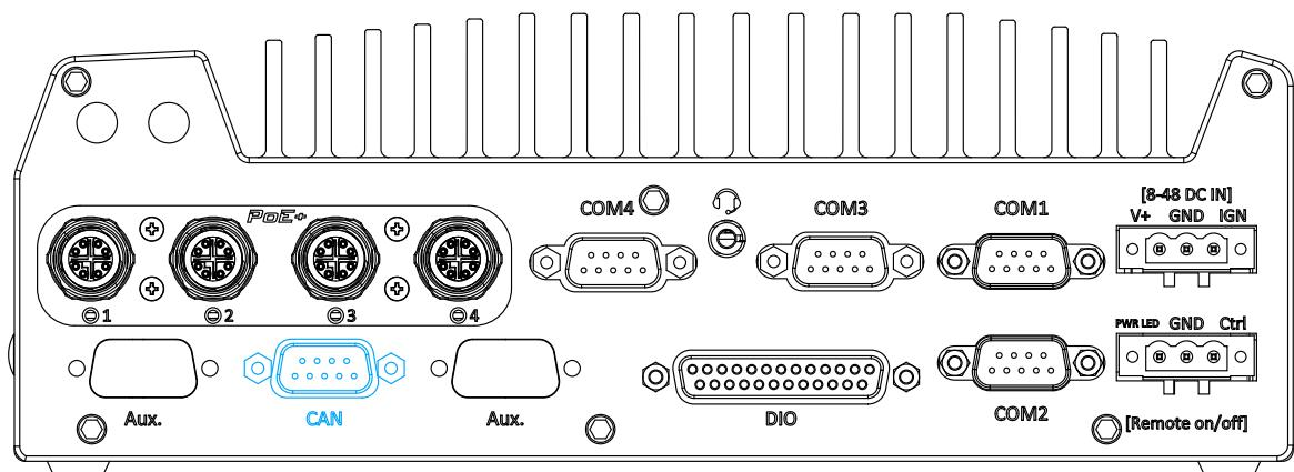
CAN bus is a robust industrial bus with a pair of differential signals and is commonly used in various industrial and in-vehicles applications. The system is equipped with a CAN bus DB9 port that is compatible with both industrial and in-vehicle applications. The CAN bus port supports CAN2.0A and CAN2.0B up to 1Mbps.
