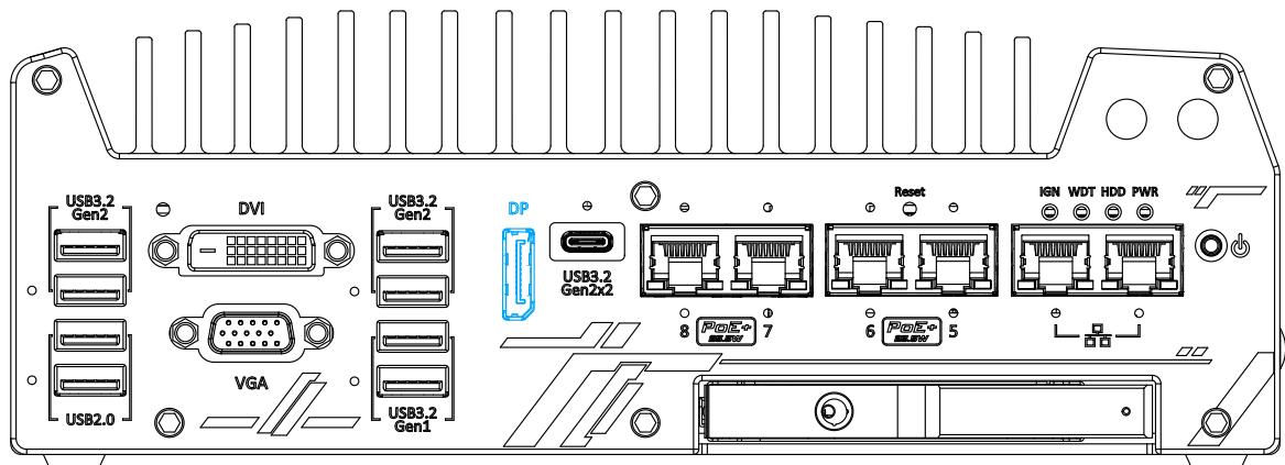
The system has a DisplayPort (DP) output which is a digital display interface that mainly connect video source and carry audio to a display device. When connecting a DP, it can deliver up to 4K UHD (4096 x 2304 @ 60Hz) in resolution. The system is designed to support passive DP adapter/cable. You can connect to other display devices using DP-to-HDMI cable or DP-to-DVI cable.
