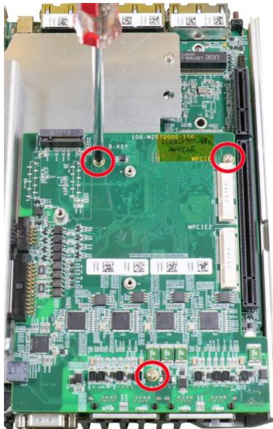
8. The The SIM slot is located underneath. The SIM socket utilizes push-push mechanism (push-to-install and push-to-retrieve).
