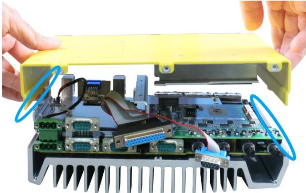
3. Install the front panel and secure screws indicated in **blue**.
