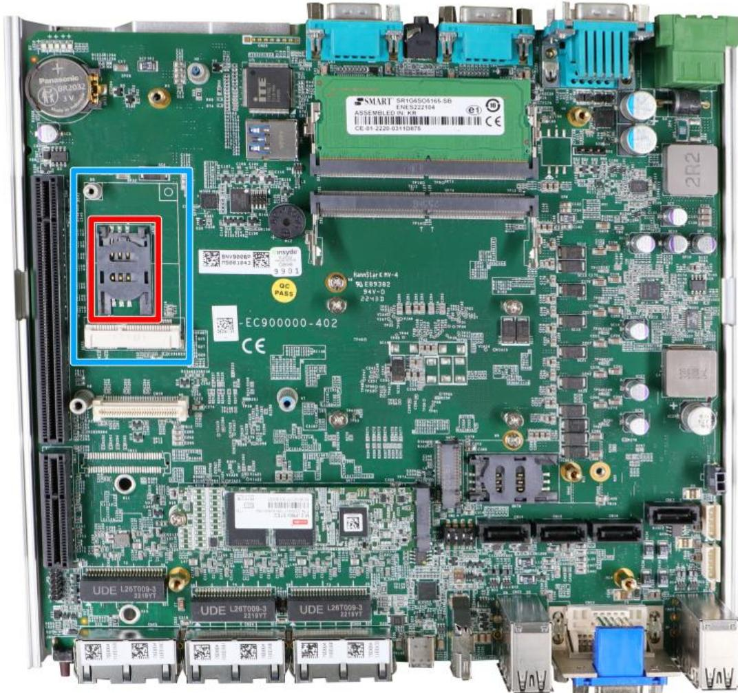
The system provides a mini-PCIe socket (indicated in **blue**) that is in compliance with mini-PCIe specification rev. 1.2. This mini-PCIe socket is designed with SIM card (slot indicated in **red**) support. With a SIM card installed, your system can access the internet via your network provider's 4G/ 3G network.
