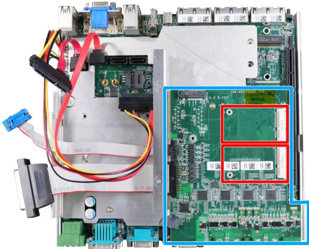
There are two additional full-size mini-PCIe sockets (indicated in **red**) available on the MezIO™ module (indicated in **blue**). They are implemented with USB signals only have better compatibility with off-the-shelf 3G/ 4G mini-PCIe modules. For customers who want to install 3G/ 4G module(s), please take advantage of these two mini-PCIe sockets and the associated SIM slots.
