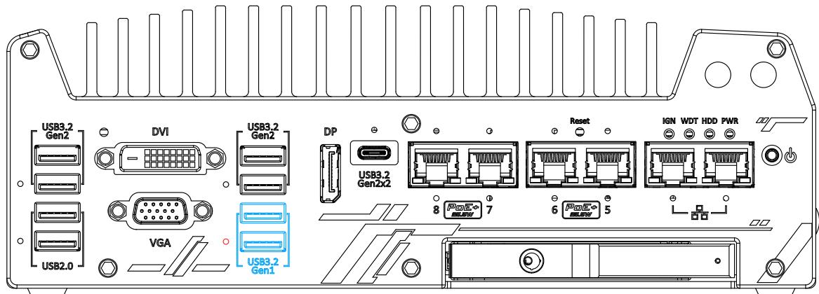
The system's USB 3.2 Gen1x1 ports (5Gbps) are implemented via native xHCI (eXtensible Host Controller Interface) controller and are backward compatible with USB 2.0, USB 1.1 and USB 1.0 devices. UEFI USB is also supported so you can use USB keyboard/mouse in UEFI shell environment. Indicated in red is a screw-lock hole for the corresponding USB port. xHCI driver is supported natively in Windows 10, therefore you do not need to install the xHCI driver prior to utilizing USB functions.
