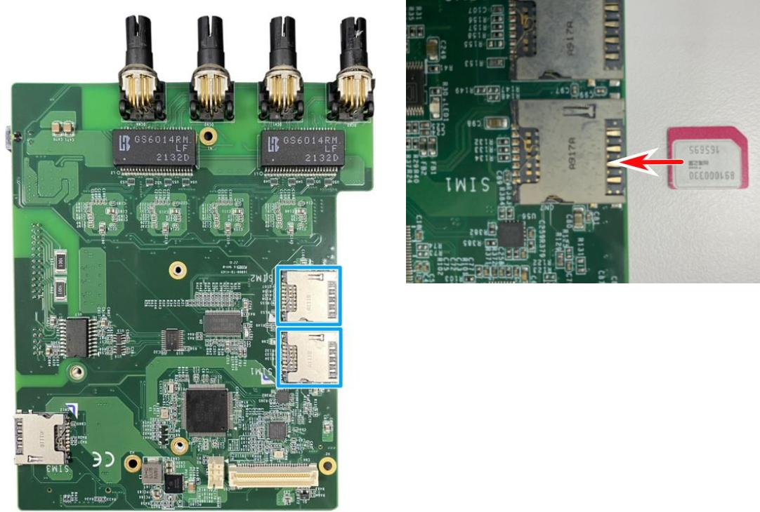
**mPCIe SIM slots underneath**
