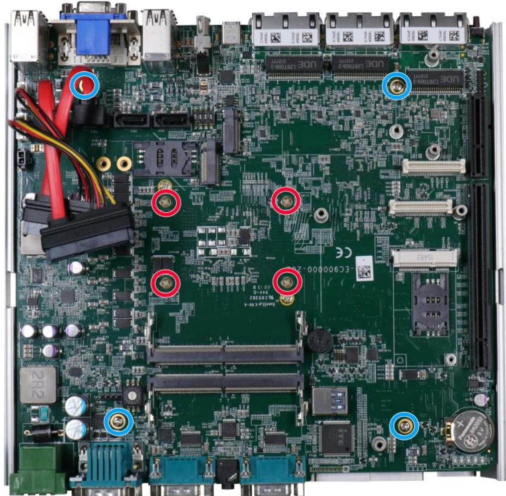
3. Remove the screws indicated once you separate the heatsink from the motherboard to remove the CPU holder.
