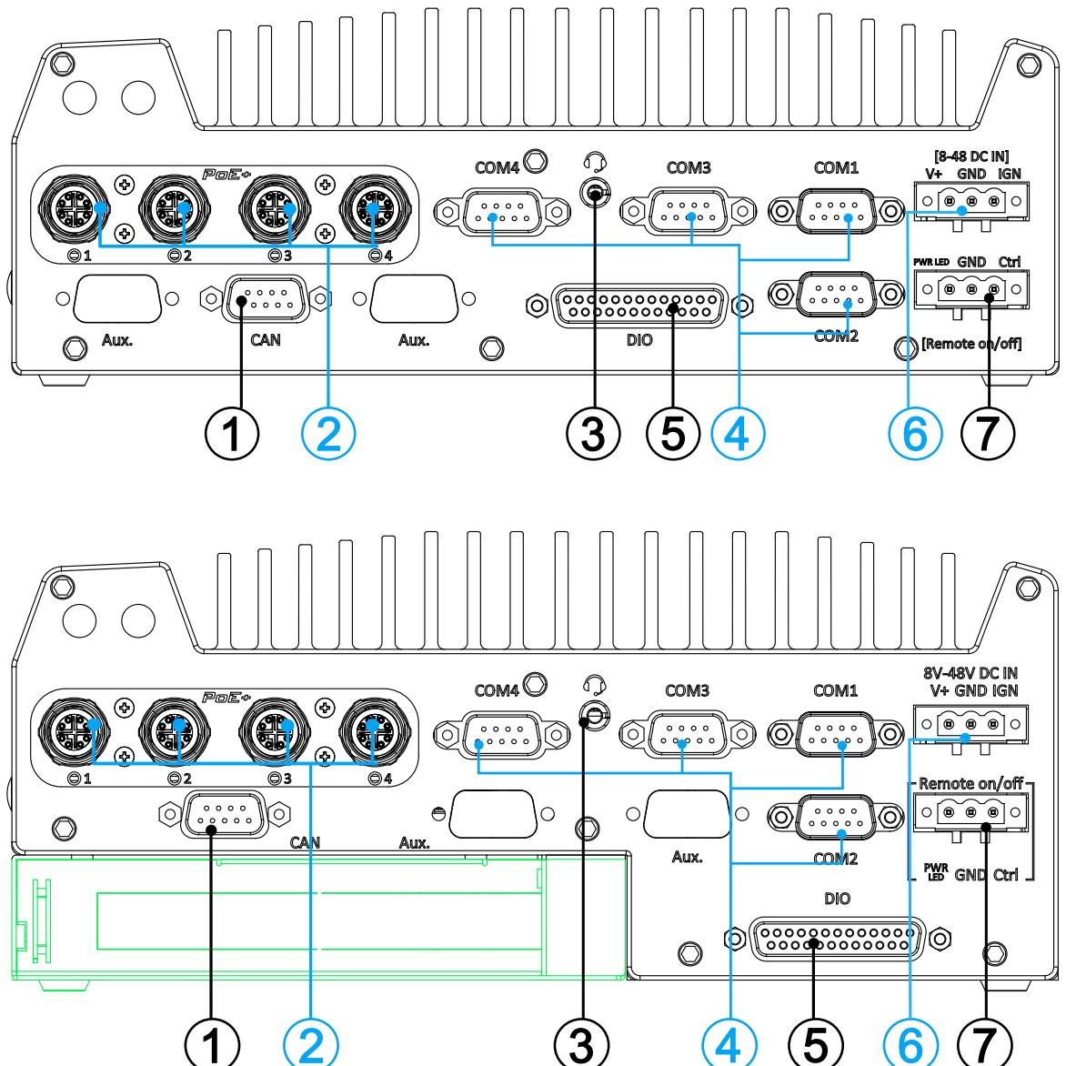
The rear panel features four RJ45 or M12 PoE ports, CAN bus, digital I/O, four COM ports, ignition control switch, 3-pin terminal and remote 3-pin on/ off control.
