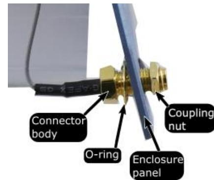
**Secure antenna to system panel**
