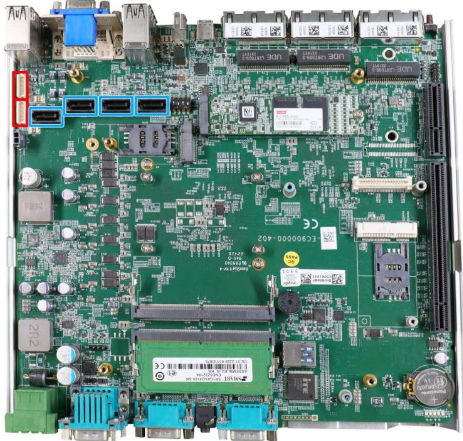
The system has SATA ports (blue) and four-pin power connectors (red). The SATA and power cables should already be connected on the motherboard so users only need to install the 2.5" SATA HDDs/ SSDs to the front hot-swappable tray(s). For Nuvo-9100VTC systems, there is also an internal drive that can be coupled to configured into RAID 0 or 1 storage.
