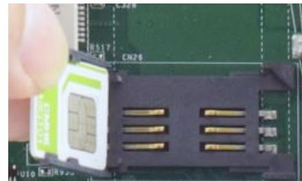
**Insert Mini-SIM card with pins
