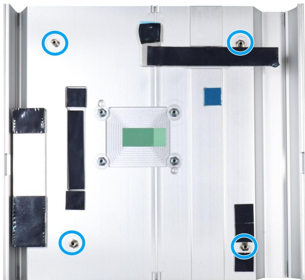
11. Once the motherboard has been installed, you're ready to secure the four screws that help the heatsink apply pressure to the CPU/ chipset die. You'll want to apply even pressure to the corners by gradually tightening each screw. Please refer to the recommended order when tightening the screws.
