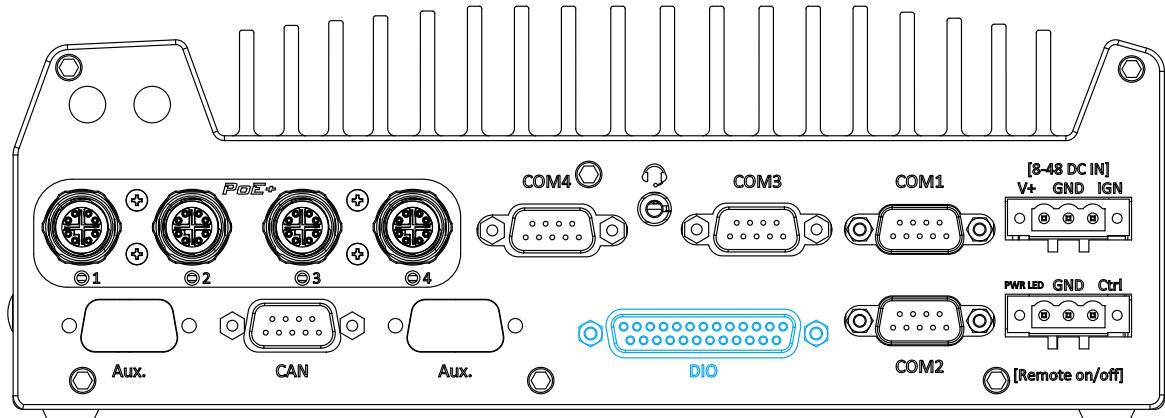
The system provides 4x isolated digital input channels and 4x isolated digital output channels. The DIO functions support polling mode I/O access and DI change-of-state interrupt. Please refer to digital I/O pin definition on the following page and [Watchdog Timer & Isolated DIO](#) for information on wiring and programming the isolated DIO channels.
