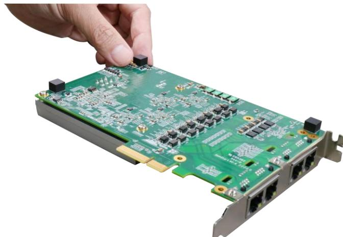
5. Remove the bezel cover (indicated in **blue circle**) and insert the card into the PCIe/ PCI slot while making sure the bezel is properly inserted into the notch and the card is secured in place with screw.
