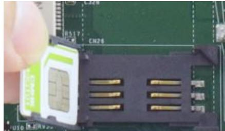
**Insert Mini-SIM card with pins**
