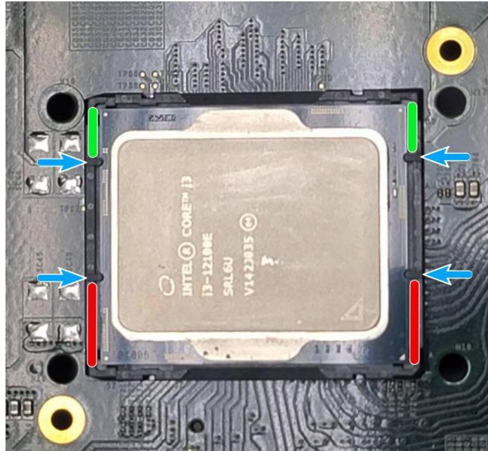
5. Locate the CPU retention bracket (holder) from the accessory box. Place the retention bracket on the CPU and hold it in place. Make sure the indicator triangle engraved on the CPU's integrated heat spreader (IHS) and the triangle indicator on the retention bracket are positioned in the same corner (indicated by **blue circles**).
