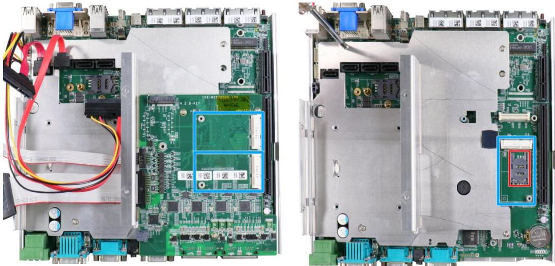
**mini-PCIe slot on MezIO™ module**
