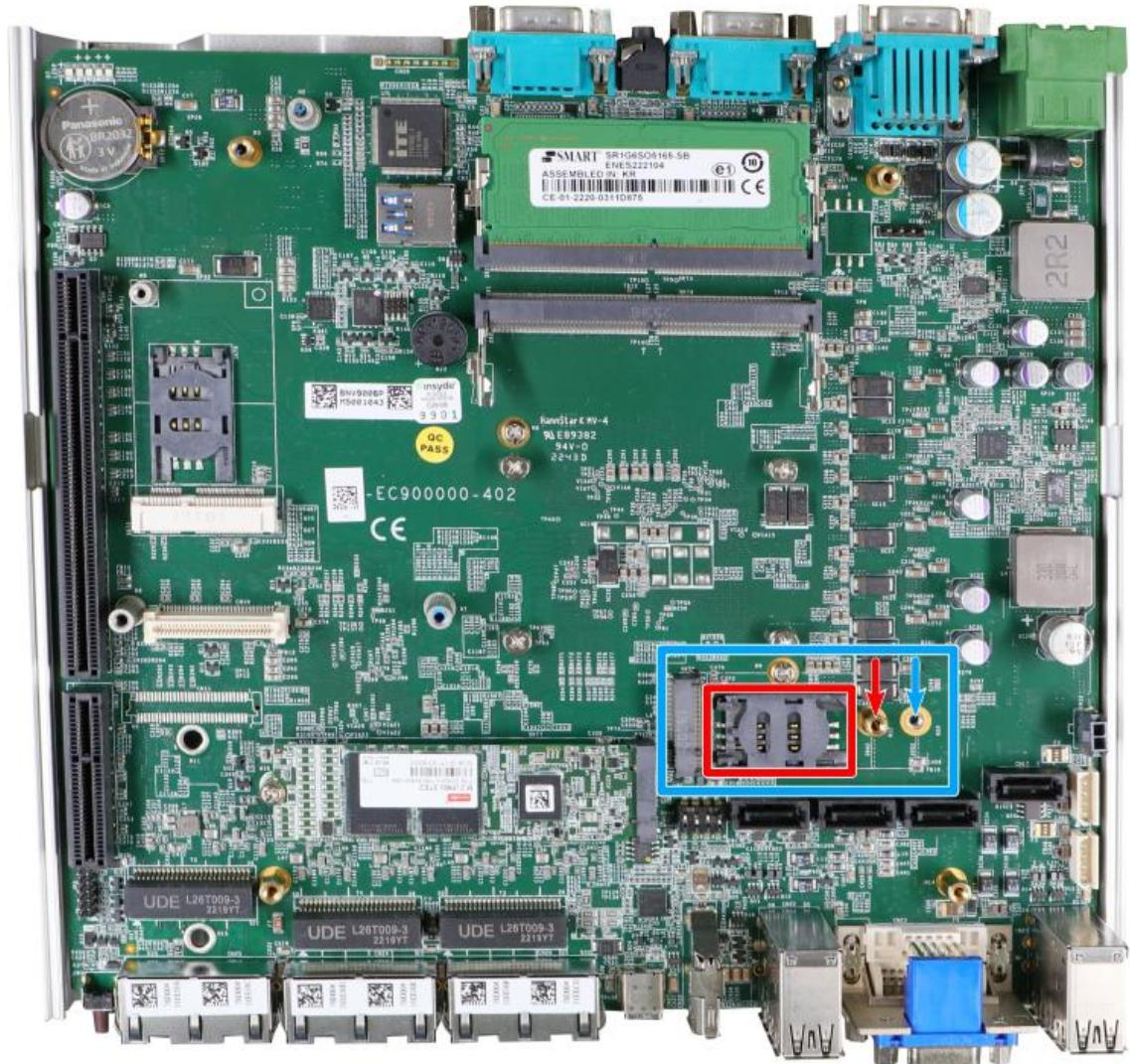
The system has an M.2 2242/ 3042/ 3052 slot (indicated in **blue rectangle**) with a 5G/ 4G SIM slot (indicated in **red rectangle**). A copper standoff is provided for you to secure onto the motherboard into the **red arrow** location for an M.2 2242/ 3042 module, or into the **blue arrow** location for an M.2 3052 module. By installing a 5G or 4G M.2 module and SIM card, you can access the internet via the provider's network.
