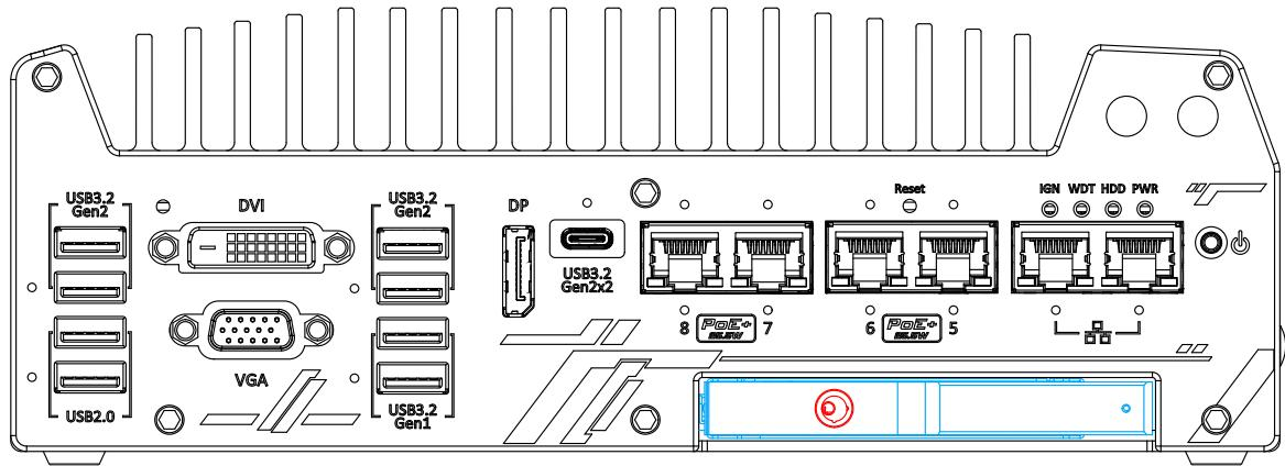
The Nuvo-9100VTC systems support an external 2.5" HDD/ SSD via a hot-swappable slot. Designed for easy access, the HDD/ SSD slot is secured by a lock (indicated in red) and it supports RAID modes 0/ 1 configuration by combining with the internal HDD/ SSD drive for OS installation (coupled with the internal HDD). To set up RAID, please refer to RAID Volume Configuration section for details.
