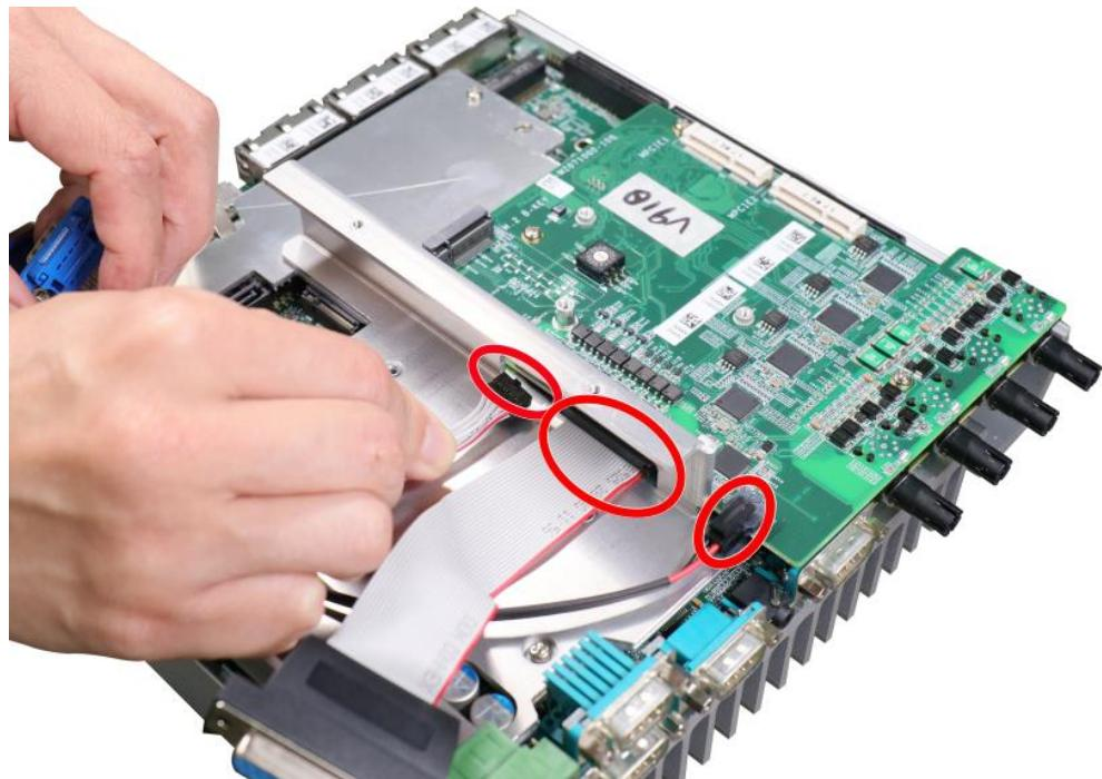
9. Remove the MezIO™ module by unscrewing the screws shown and gently lift to separate it from the motherboard.
