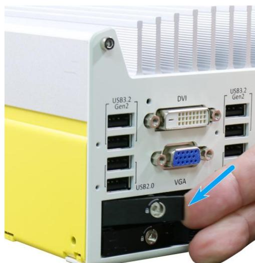
2. With the label side facing upward, insert the SATA connector side of the 2.5" HDD/ SSD into the slot first. You may feel resistance when the SATA connectors meet, push it in firmly until the 2.5" HDD/ SSD is fully inserted into the slot.
