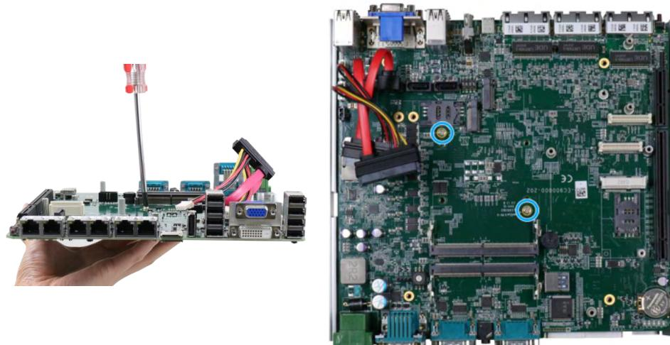
**Hold CPU bracket firmly and turn
