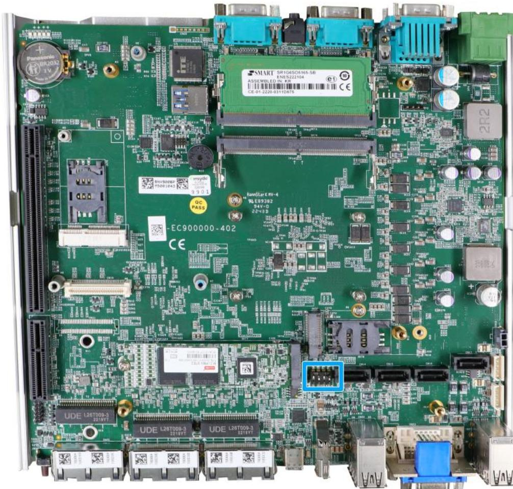
The DIP switch (indicated in blue) is reserved for manufacturing/ engineering purposes and should already be configured out of the factory. The table below shows the system default DIP switch settings for reference purposes.
